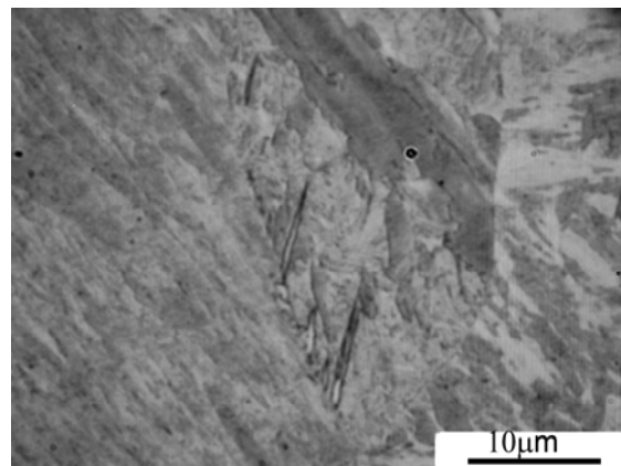
d) OM/WSF-Onset / Ti-V-N steel /450°C/ 10s/1000X
