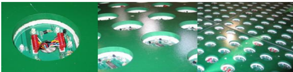
Figure 5. Installation of LED in the solar road panel SR1
