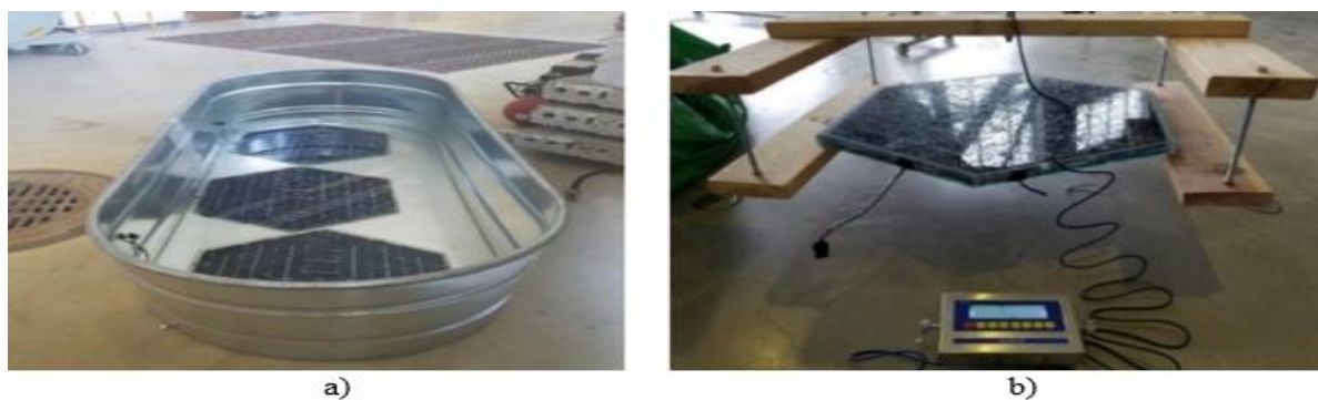
Figure 14. Moisture resistance testing of SR3 solar road panels: a) Immersion in water, b) Measuring weight after immersion in water [17]
