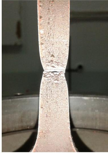
Figure A.2: Typical coupon specimen failure.
