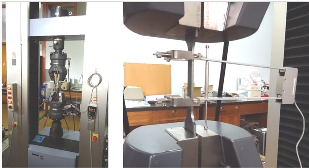
Figure A.1: Universal Testing Machine Shimadzu AG-Xplus and extensometer with an initial length of 50 mm.
