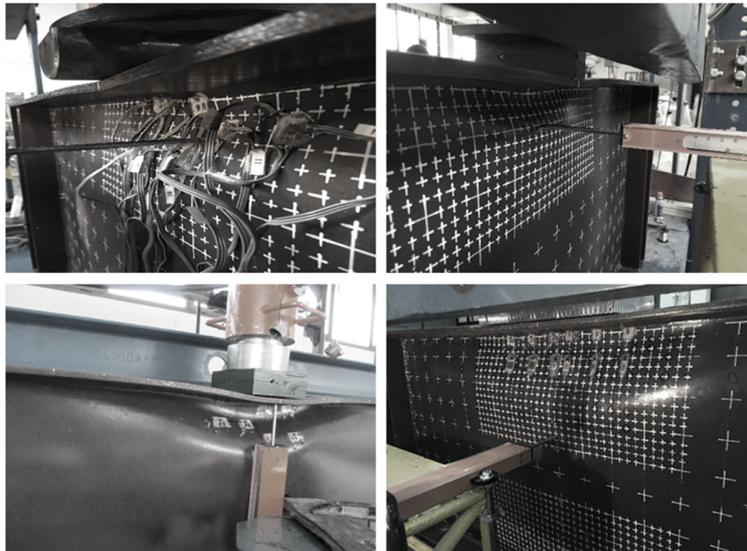
Figure 3.15: Web and flange deformation for applied forces near the ultimate strength for girders (clockwise from top left) B16, B14, B11, and B15.
