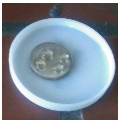
Figure 3. Hydrophobic effect on the copper coated with silver in combination with a self-assembled hydrophobic perfluorodecyltrichlorosilane (FDTS) layer.
