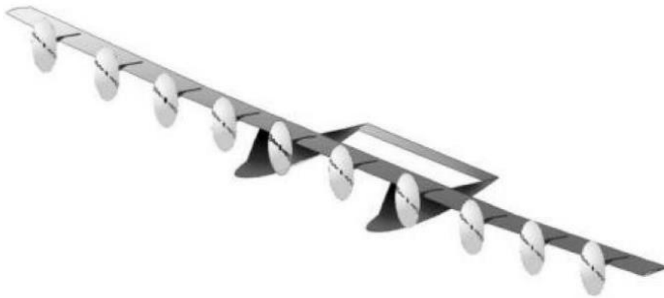
Figure 3- 9: An artist's impression of the braced wing concept [71]
