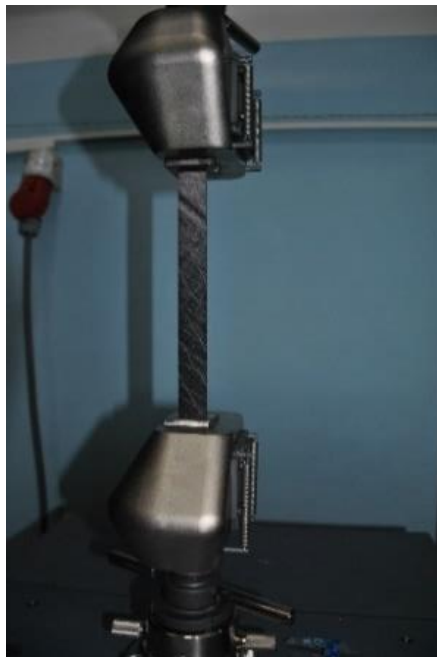
Figure 7- 17: Test sample prepared for testing in Shimadzu tensile testing machine [123]
