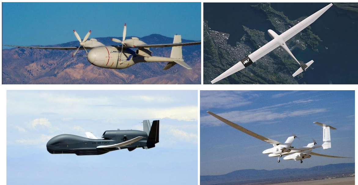
Figure 3- 1: High- altitude long endurance drones: the Phantom Eye, the Global Observer, the RQ-4B Global Hawk, the Theseus aircraft by Aurora Flight Sciences Corporation [62][63][64][65]
