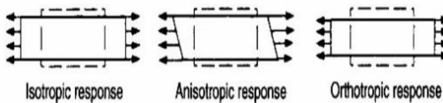
Figure 7- 16: Behavior of isotropic, anisotropic and orthotropic materials under the tensile force
