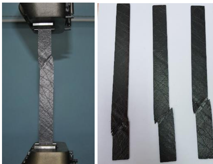
Figure 7- 20: Sample type 1 and their fracture positions [123]
