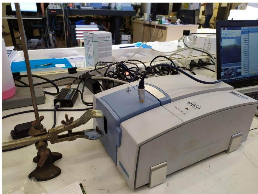
Figure 31: Bruker Optic Alpha-R portable interferometer, INFN National Laboratory of Frascati (photo A. Petrović)
