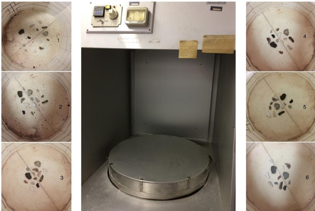
Figure 96: Experimental oven at LTFAPA (Sapienza University of Rome) and six phases of heating – the position of the tools inside the oven (photo A. Petrović)
