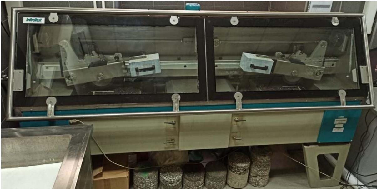
**Figure 4.25** *Wheel tracking device*
