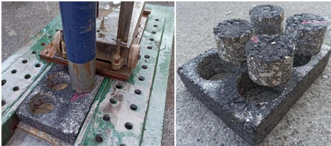
*Figure 4.18 Preparation of testing specimens for fatigue resistance determination*
