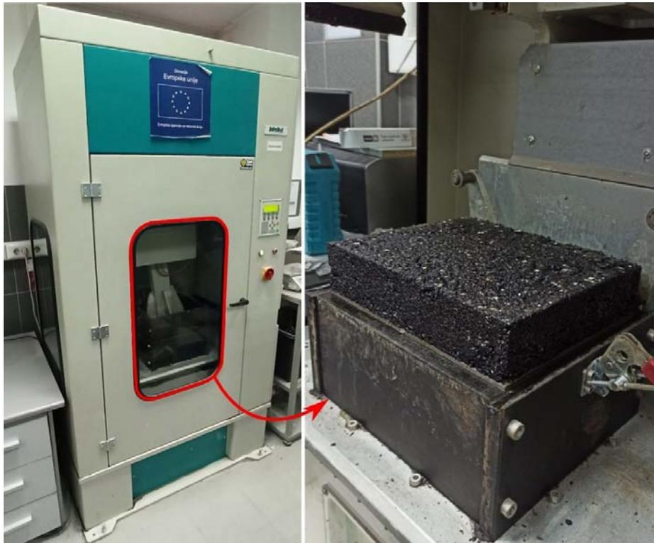
*Figure 4.17 Slab compactor*
