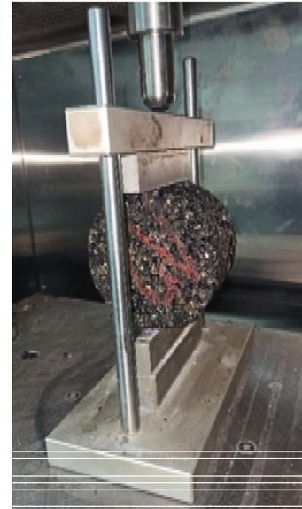
Figure 4.19 The testing head configuration
