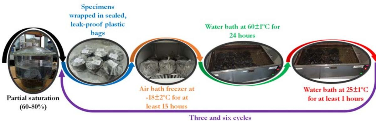
Figure 4.20 Procedure of specimens' preparation for freeze-thaw resistance test
