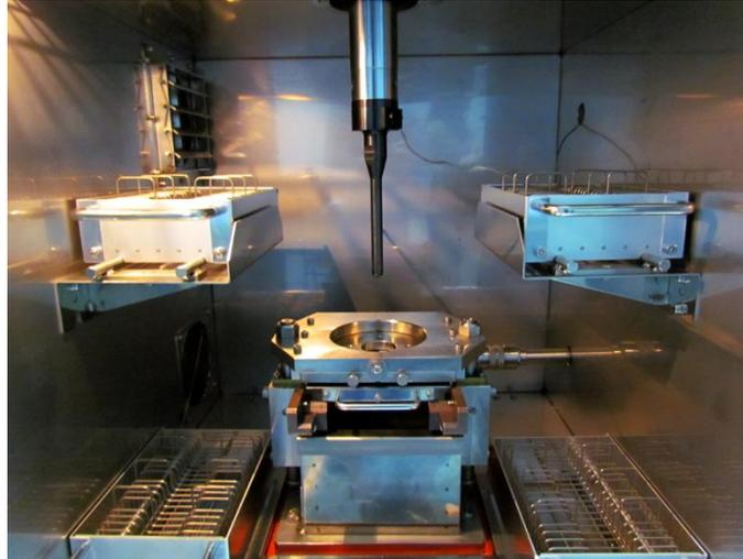
*Figure 10 The specimen for high speed impact testing in the testing machine after the impact.*
