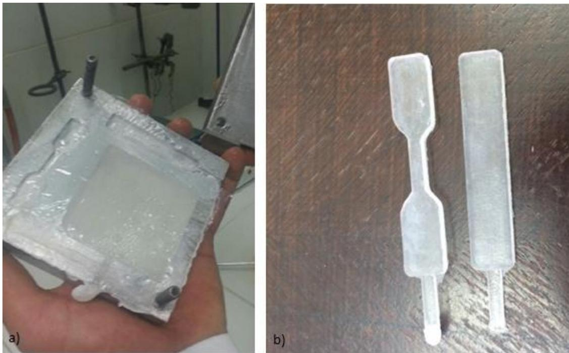
***Figure 12 a) The mold for sample preparation showing the forms for preparation of the sample for tensile testing, for 3 point bending testing and for high speed impact testing, b) The specimens for tensile testing and 3 point bending testing just after being prepared.***
