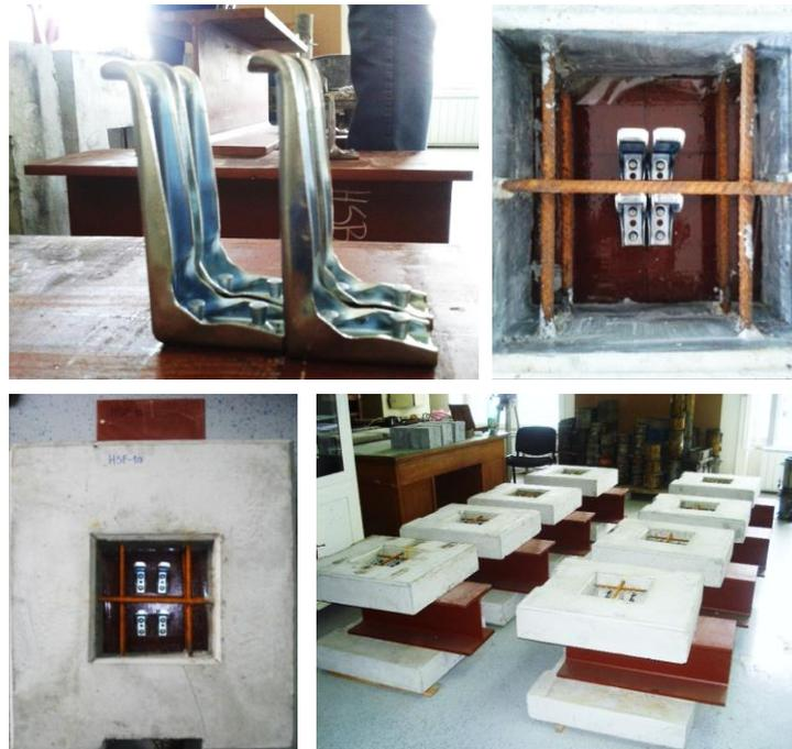
**Figure 4.5.** *Push-out specimens assembling*
