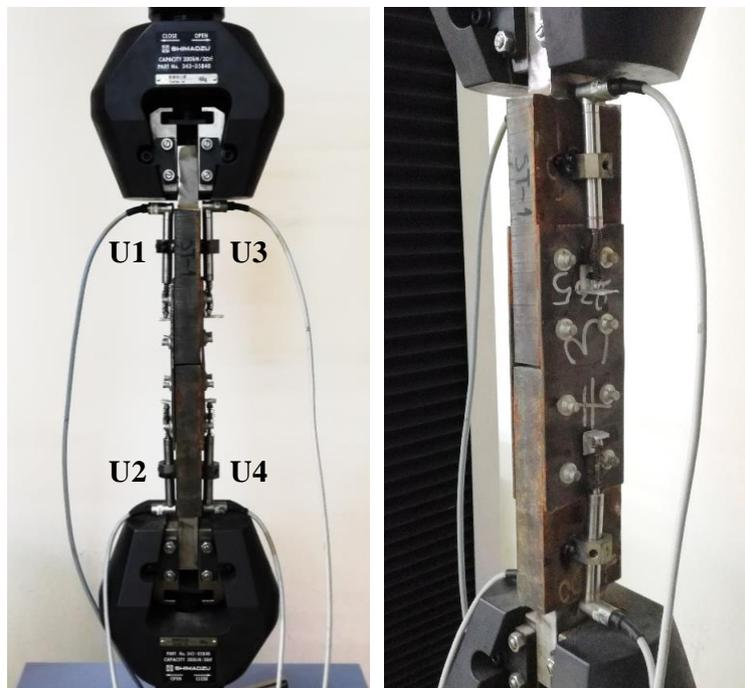
**Figure 4.31.** Examination of shear test specimens - ST
