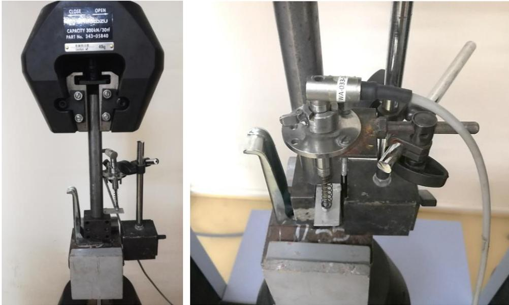
*Figure 4.32. Examination of tension test specimens - TT*
