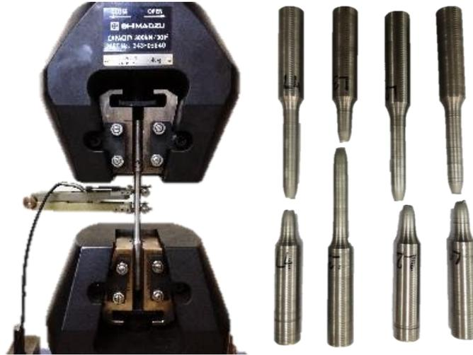
*a) tensile tests of round coupons*
