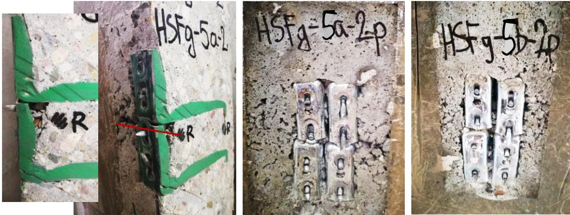
**Figure B.3.** Installation mistakes - HSFg5-2 specimen
