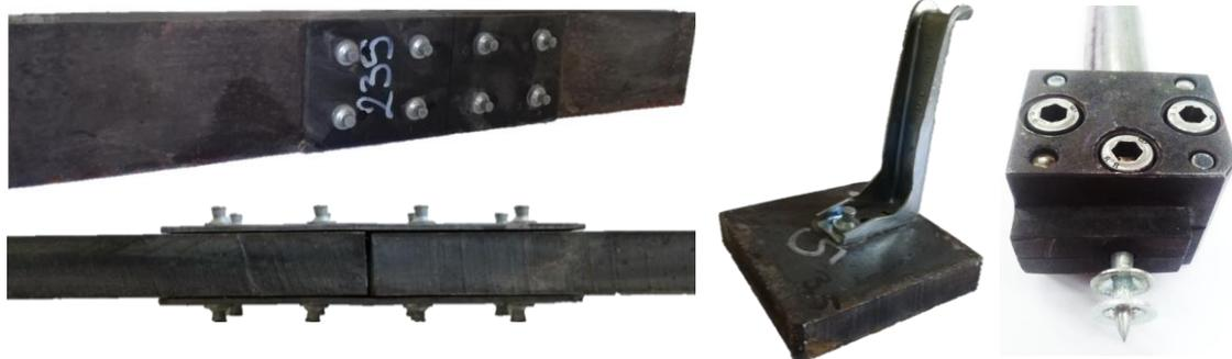
*a) shear test specimens - ST*
