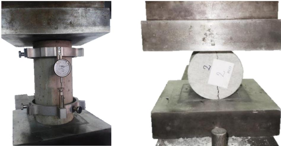
a) elastic modulus examination      b) splitting tensile strength examination
