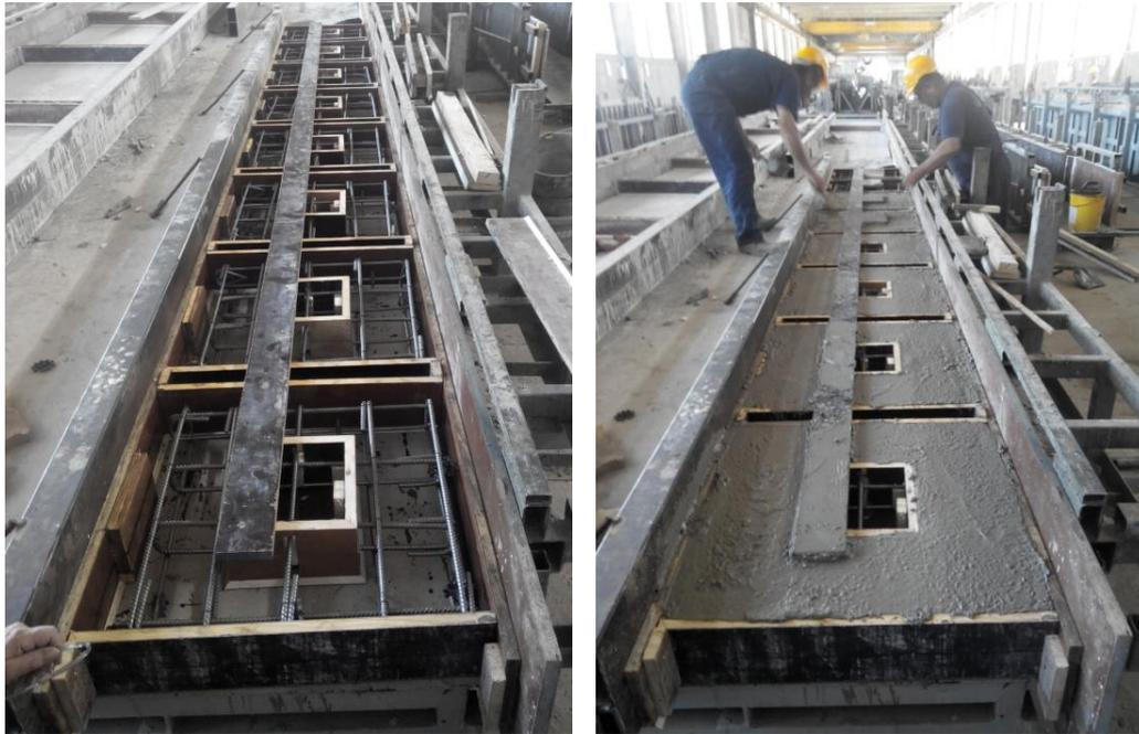
**Figure 4.4.** Prefabrication of concrete slabs in “ASA IBELIK” concrete plant
