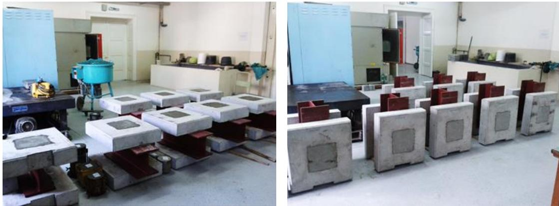
*a) specimens after concreting*
