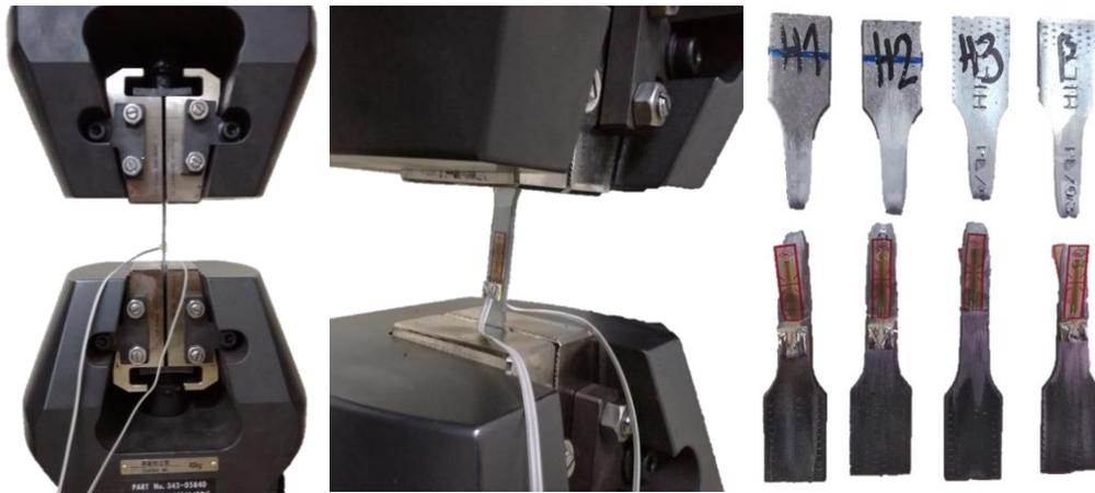
*b) tensile tests of flat coupons*
