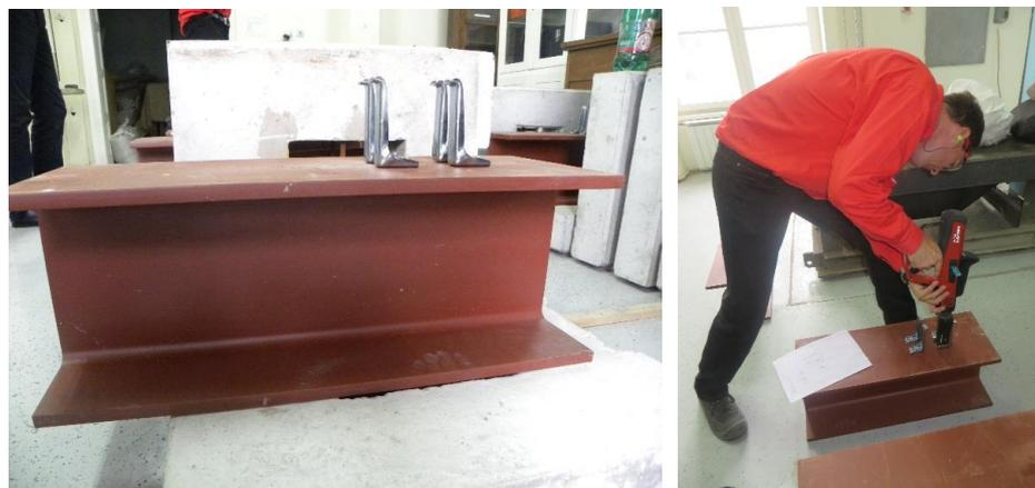
**Figure 4.6.** *Installation of X-ENP-21 HVB cartridge fired pins*
