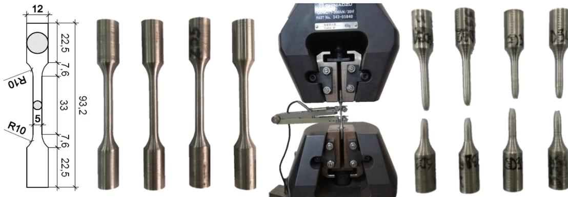
a) base plate tensile test coupons
