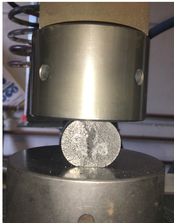
Figure 5.13. Experimental setup of Brazilian test
