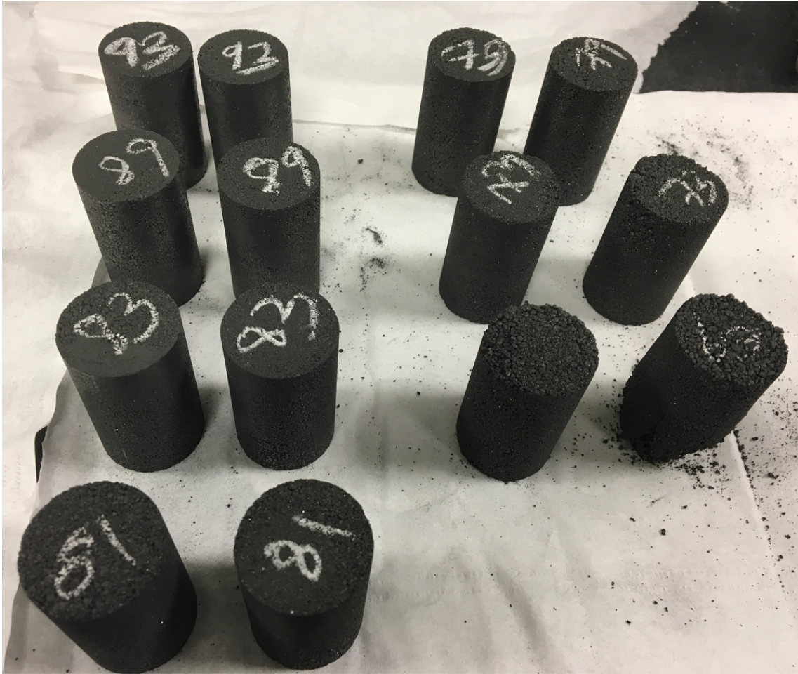
Figure 5.3. Prepared samples for crush tests
