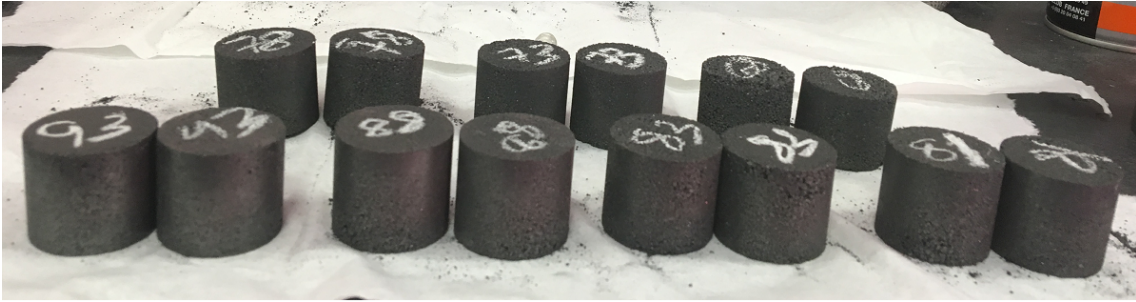
Figure 5.5. Prepared samples for Brazilian tests
