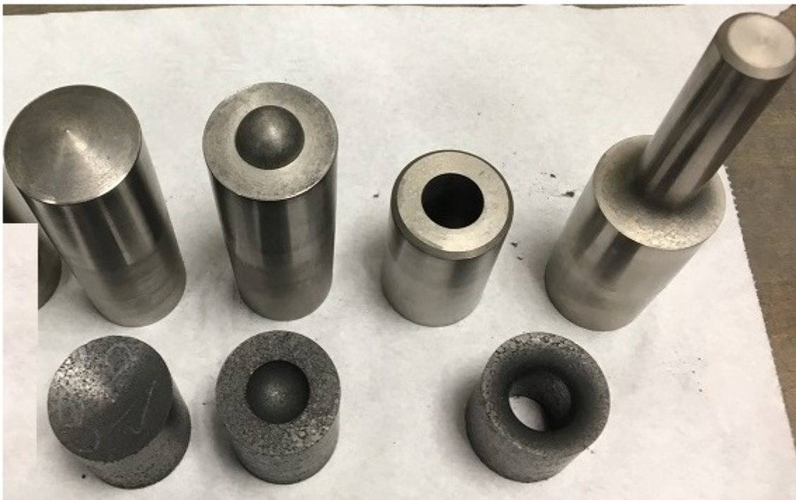
Figure 5.50. Samples made from alumina-graphite powder along with the required punches to produce configurations -5 to -7 (Left to Right)
