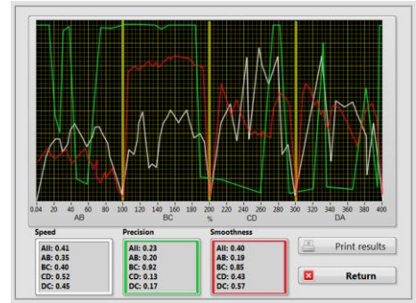
Fig 4. User friendly software interface. Main window provides intuitive commands for the testing procedure and the score (top panel). Individual metrics can be examined by the operator in the "Detailed results" window (bottom panel).
