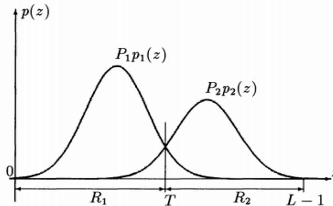
Figure (4.10) Gray-level probability density functions of two regions in an image.
