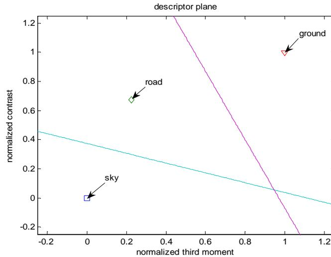
Figure 5.18 The classification used min Euclidean distance.
