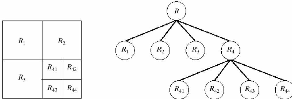
Figure 3.3 partitioned image and its corresponding quad tree.
