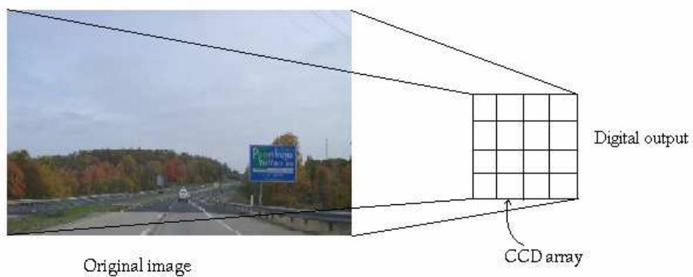
Figure 2.1 capturing an image with CCD camera.
