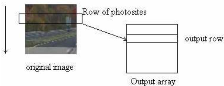
Figure 2.2 capturing an image with CCD scanner.
