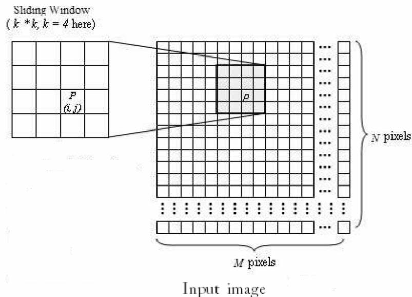
Fig (4.9): Texture Feature Extraction for pixel  $p(i, j)$  (window size is  $4 \times 4$ )
