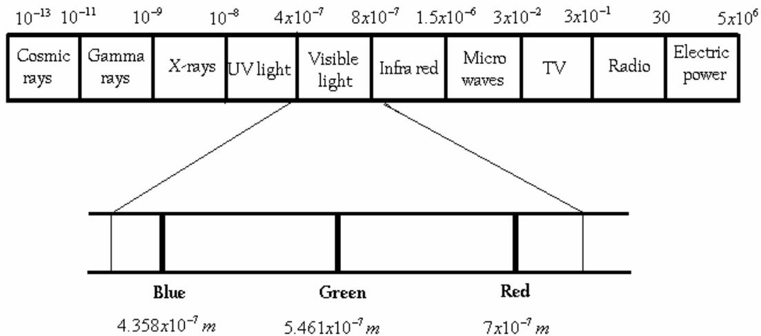
Figure 2.3 the electromagnetic spectrum.
