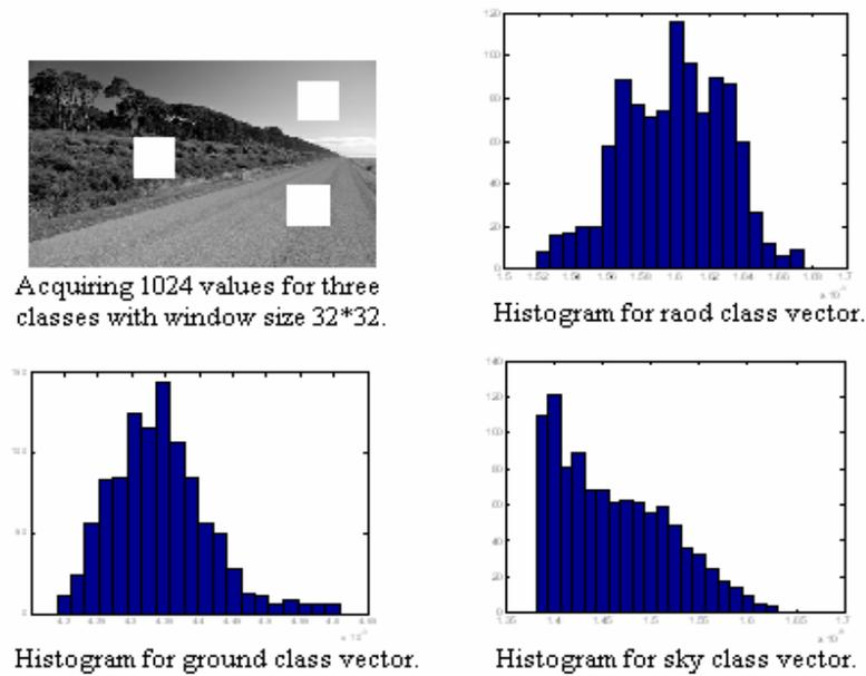
Figure 5.9 Co-occurrence descriptor (contrast) reading 1024 values by three windows size 32\*32 and their histograms.
