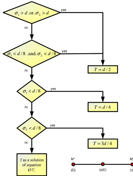
Figure 5.17 Flowchart for specification of the threshold.
