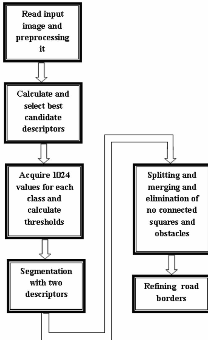
Figure 1.1 Algorithm block diagram
