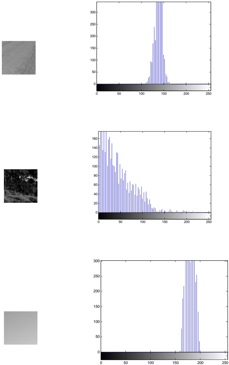
Figure 3.1 Histogram of three different sub- images( low contrast, dark, light)
