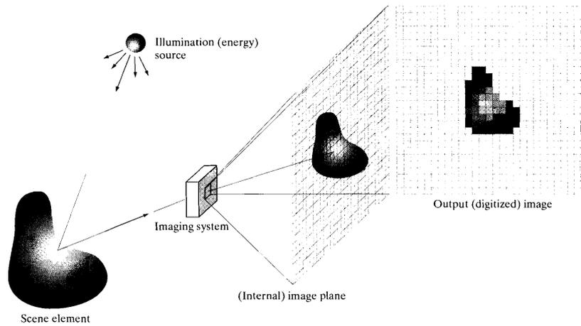
Figure 2.4 an example of the digital image acquisition process
