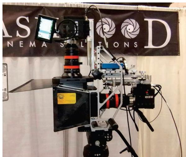
**Slika 2.13:** 3D BX4 stereoskopski *beam-splitter* sa RED *Epic* kamerama, (R. Zone, Spatial plasticity: Dual-camera configurations and variable interaxial, [61]).
