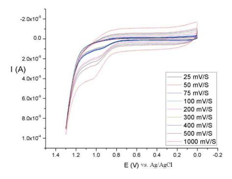
**Figure 14**. Cyclic voltammograms of H<sub>2</sub>(acac phacac en)
