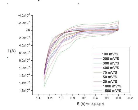
**Figure 12**. Cyclic voltammograms of  $H_2(acac_2 en)$
