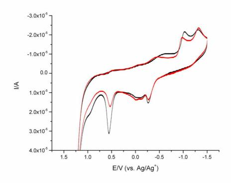
**Figure 38.** Voltammograms of  $[Cu(acac_2 en)]$  (black) and  $[Cu(acac_2 pn)]$  (red),0.1 V s<sup>-1</sup>
