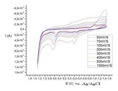
**Figure 23.** Cyclic voltammograms of [Cu(*acacphacac en*)]
