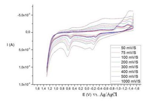
**Figure 26.** Cyclic voltammograms of [Cu(*acac*<sub>2</sub> *pn*)]
