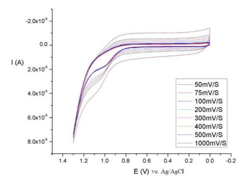
**Figure 15**. Cyclic voltammograms of  $H_2(acac_2 pn)$
