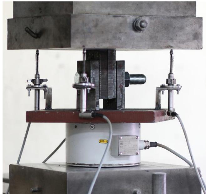
**Fig. 4.34** Shear test of the bolt - test set-up.
