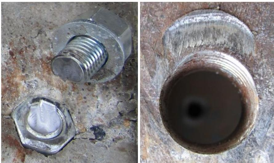
**Fig. 7.10** Characteristic failure of bolt by shear and nut and thread penetration.
