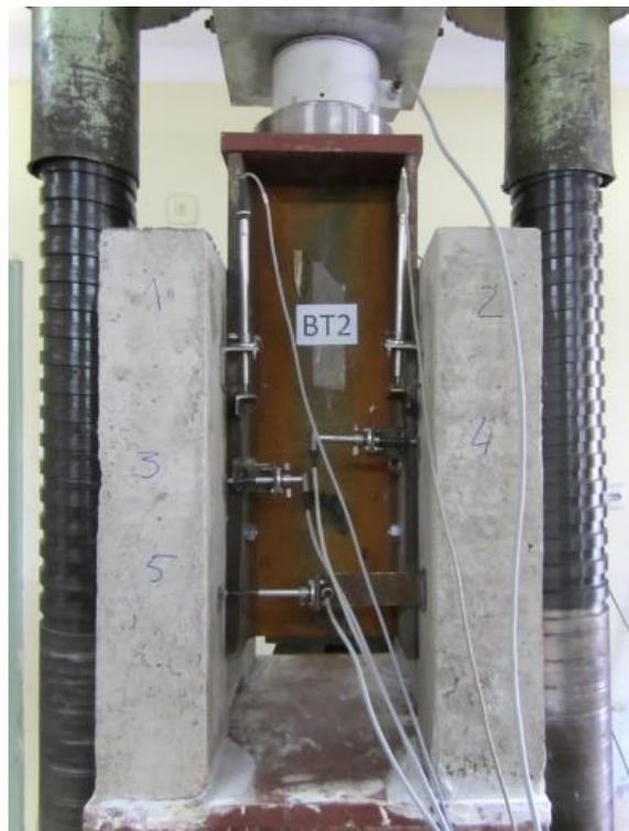
**Fig. 4.20** Specimen in a testing frame with hydraulic jack.
