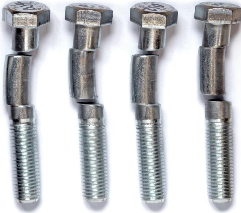
**Fig. 4.35** Bolts after failure.
