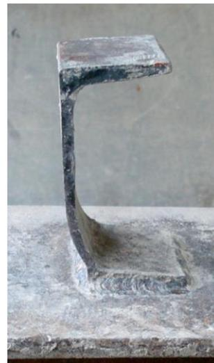
**Fig. 2.17** Channel shear connectors [Maleki and Bagheri, 2008].
