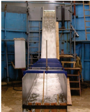
Figure 1. Scale model of the section of the weir with the stepped spillway of the Bogovina dam [3, 4]
