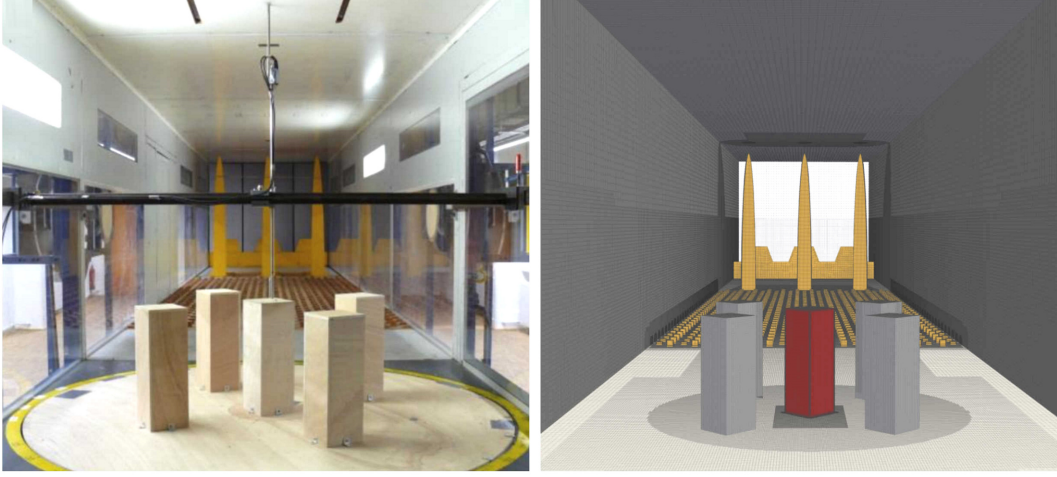
Figure 4.5. Wind tunnel test section: experimental setup of the group configuration in the ABL wind tunnel of the Ruhr-University Bochum, Germany, on the left and computational domain for the group configuration related to LES on the right, adapted from [42, 102].
