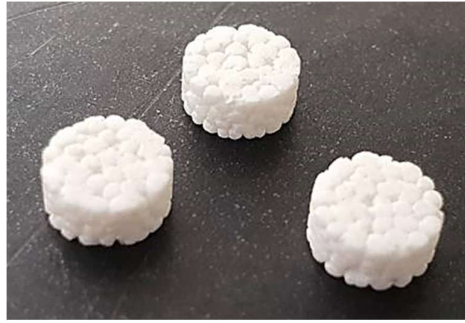
Fig. 8. The appearance of the compacts prepared from P-series samples (diameter 6 mm)
