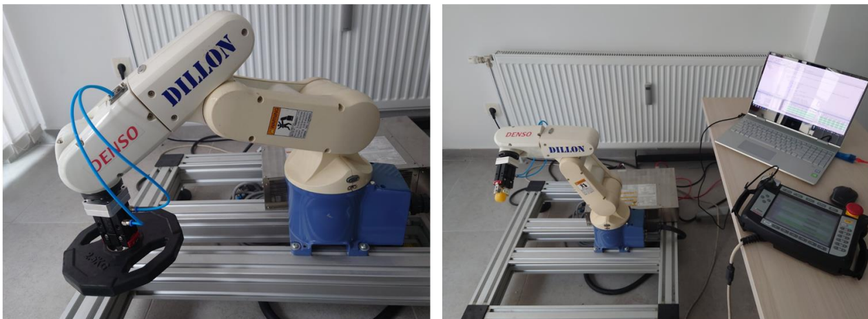
Figure 43. Measurement setups [59]. (left) Load manipulation contact task. (right) Snap-fit assembly contact task.
