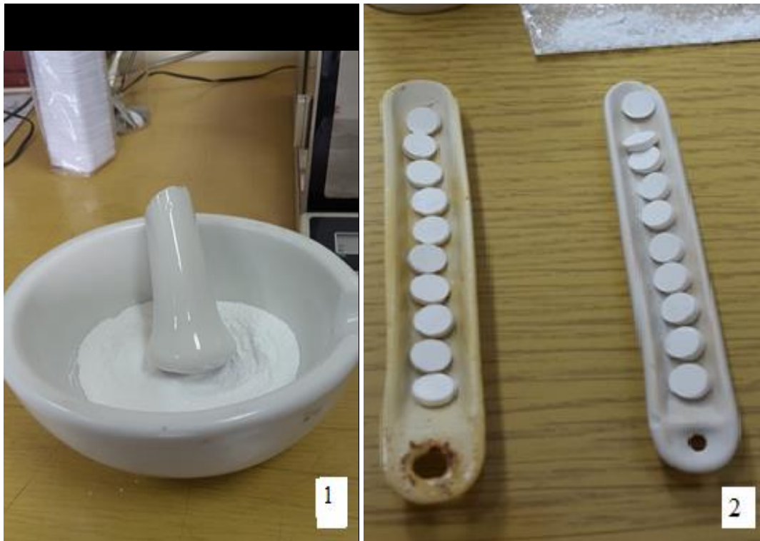
Figure 16. Photographs of 1) The composite powder. 2) Insert green samples.
