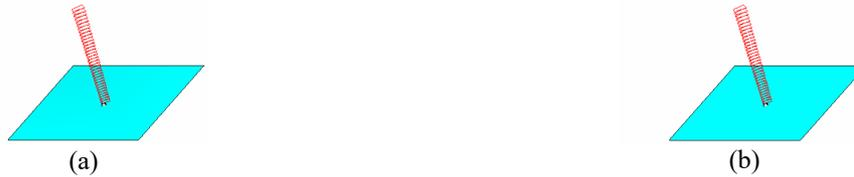
Figure 5.11. WIPL-D models that correspond to the (a) vertical scenario and (b) horizontal scenario.
