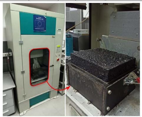
Figure 4.17 Slab compactor
