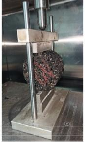
Figure 4.19 The testing head configuration
