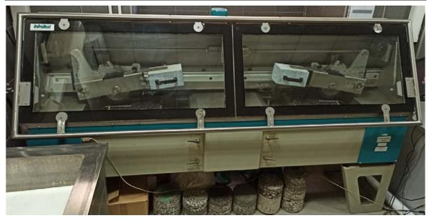
Figure 4.25 Wheel tracking device
