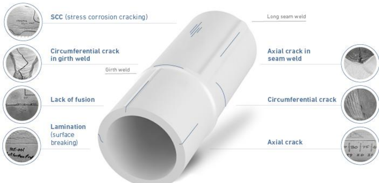
Figure 2-11: Some examples of pipeline cracks
