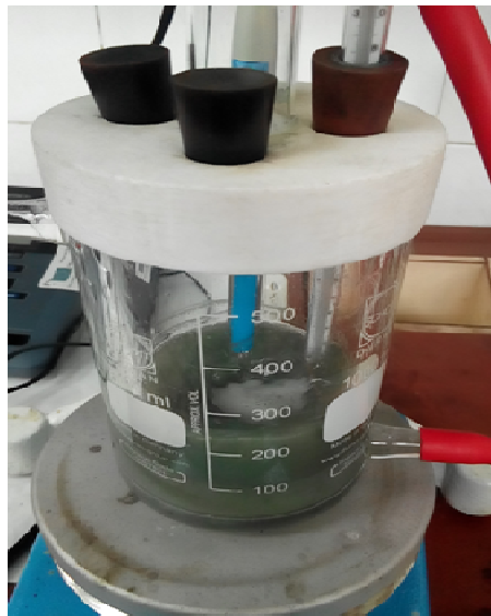
Slika 5.53. Eksperiment luženja halkopirita u rastvoru 3,0 \text{ mol/dm}^3 \text{ H}_2\text{SO}_4 + 2,0 \text{ mol/dm}^3 \text{ H}_2\text{O}_2 + 3,0 \text{ mol/dm}^3 \text{ CH}_3\text{OH} , 40^\circ\text{C} , 400 \text{ min}^{-1} , 30. minut reakcije
