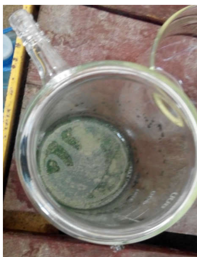
Slika 5.26. Suspenzija nakon 120 minuta luženja (Uslovi: 3,0 \text{ mol/dm}^3 \text{ H}_2\text{SO}_4 + 2,0 \text{ mol/dm}^3 \text{ H}_2\text{O}_2 , 40°C, 400 \text{ min}^{-1} )
