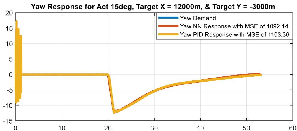
Figure 157 - Comparison of Yaw Response Between LNNA and PID for Max Actuator Deflection of 15deg and Target Located at  $X_t = 12000m$  and  $Y_t = -3000m$
