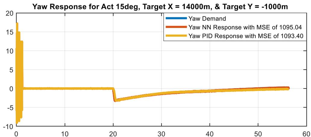
Figure 169 - Comparison of Yaw Response Between LNNA and PID for Max Actuator Deflection of 15deg and Target Located at  $X_t = 14000m$  and  $Y_t = -1000m$
