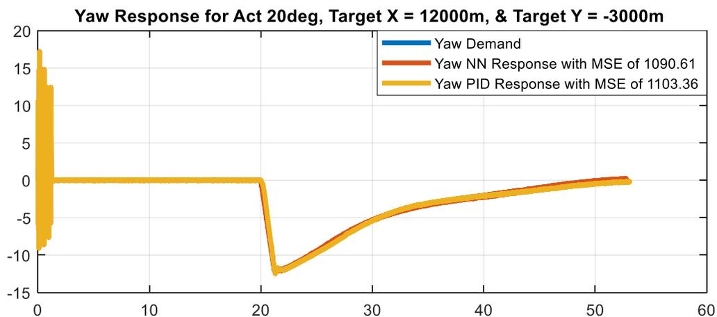
Figure 215 - Comparison of Yaw Response Between LNNA and PID for Max Actuator Deflection of 20deg and Target Located at  $X_t = 12000m$  and  $Y_t = -3000m$
