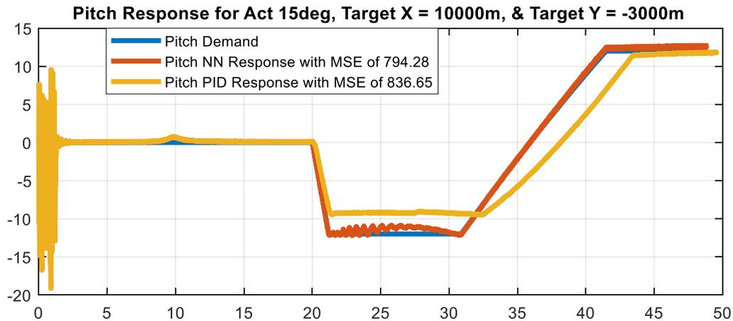
Figure 138 - Comparison of Pitch Response Between LNNA and PID for Max Actuator Deflection of 15deg and Target Located at  $X_t = 10000m$  and  $Y_t = -3000m$
