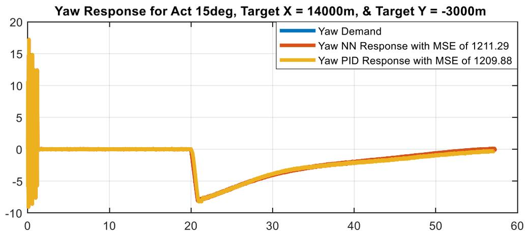
Figure 175 - Comparison of Yaw Response Between LNNA and PID for Max Actuator Deflection of 15deg and Target Located at  $X_t = 14000m$  and  $Y_t = -3000m$
