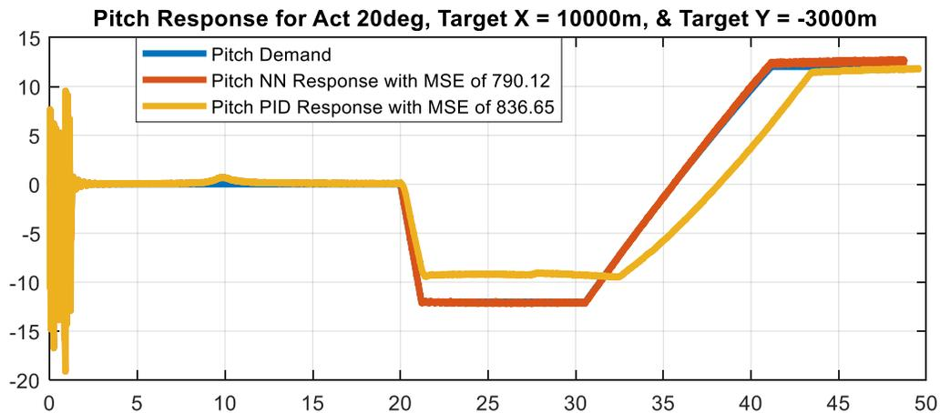
Figure 196 - Comparison of Pitch Response Between LNNA and PID for Max Actuator Deflection of 20deg and Target Located at  $X_t = 10000m$  and  $Y_t = -3000m$
