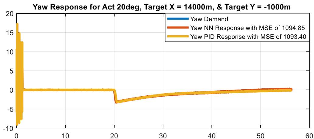
Figure 227 - Comparison of Yaw Response Between LNNA and PID for Max Actuator Deflection of 20deg and Target Located at  $X_t = 14000m$  and  $Y_t = -1000m$
