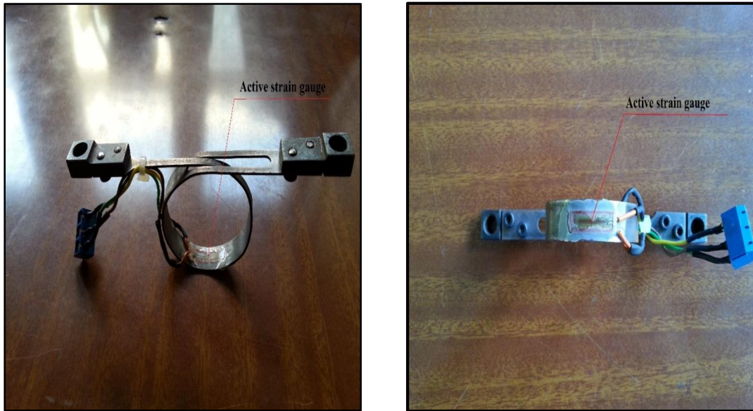
Figure 5.3 Two active stain gauges on CLD
