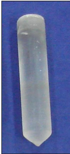
**Figure 36. Photographs of Bridgman-grown CaF<sub>2</sub> single crystal.**
