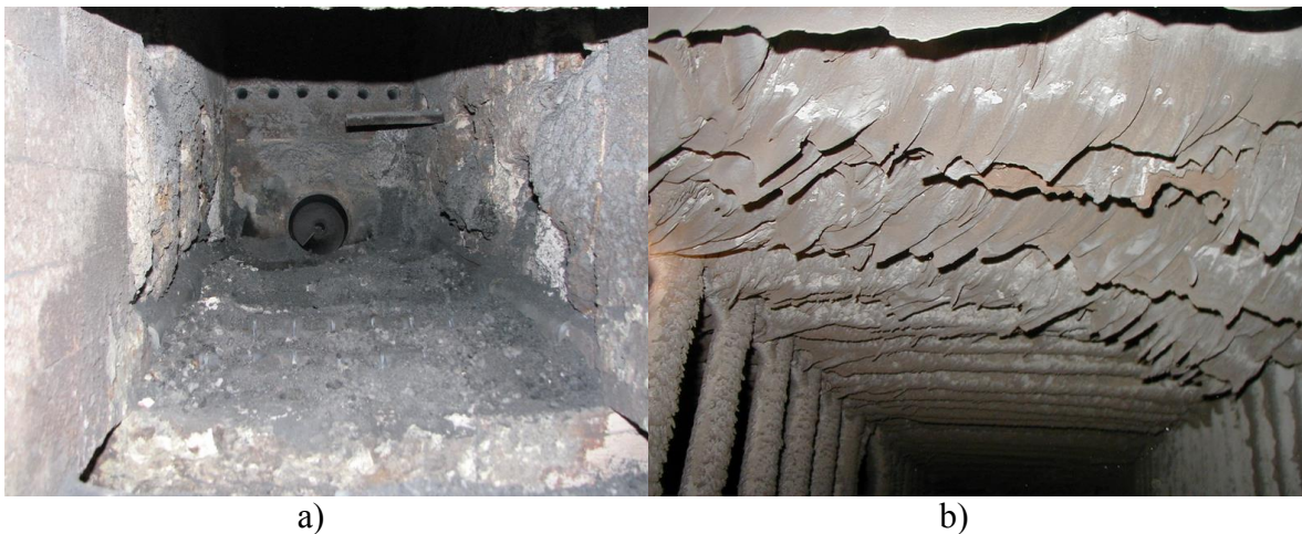
Figure 5.11 Molten ash agglomerations formed during the combustion of herbaceous fuels (a) and Hard super heater deposits in a waste wood fired boiler (b) [212]
