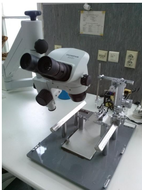
Figure 8. Stereotaxic frame and stereomicroscope
