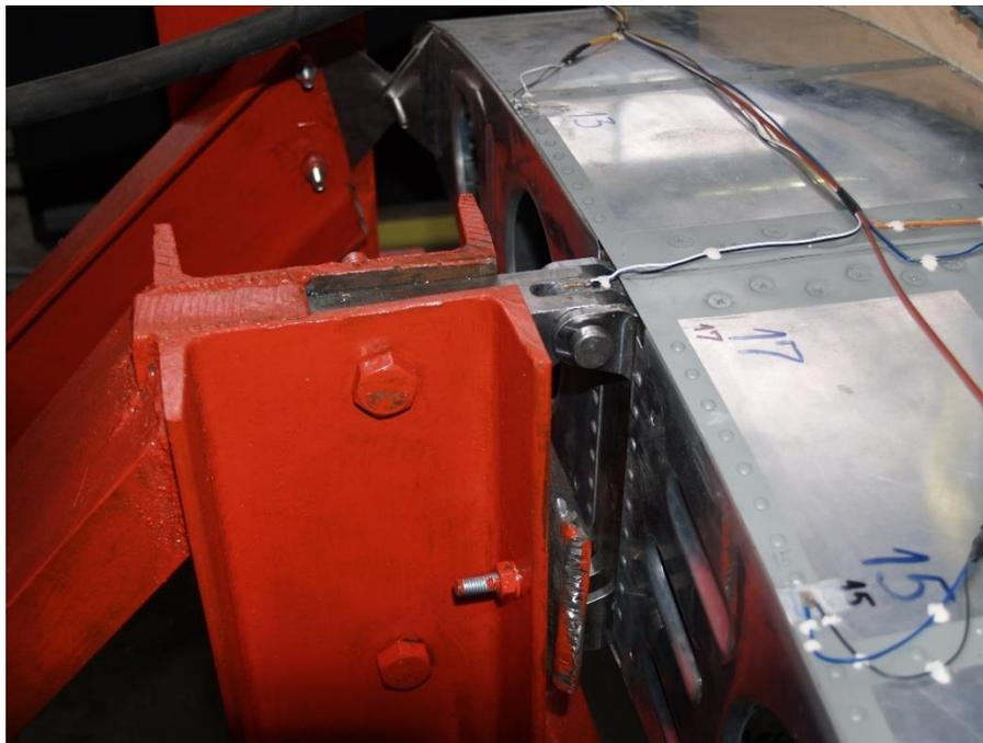
Figure 6.17 Whiffle-tree is not introducing the force on the 11<sup>th</sup> rib
