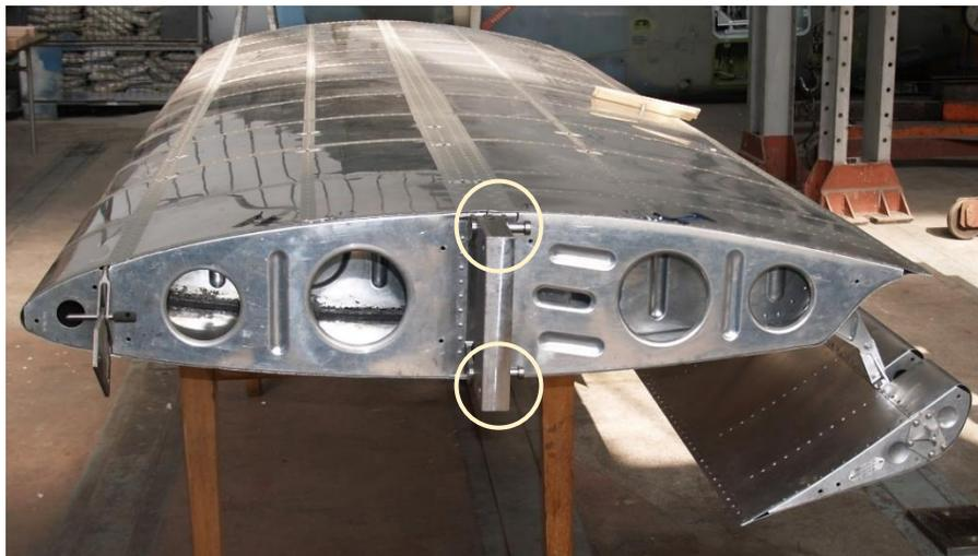
Figure 6.3 Rib number 11 and pins (circled) used to connect the central spar to steel plate
