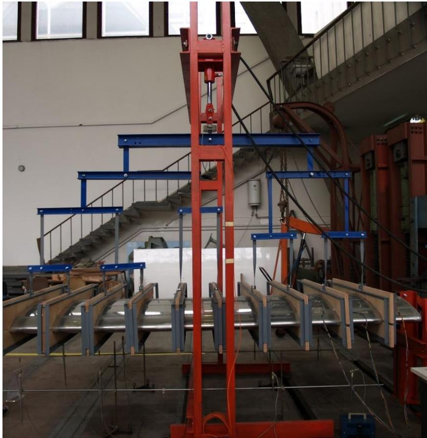
Figure 6.18 Test assembly for the light aerobatic aircraft wing
