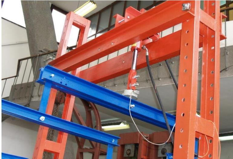
Figure 6.10 Hydraulic jack (with force transducer) used to apply loads on the wing
