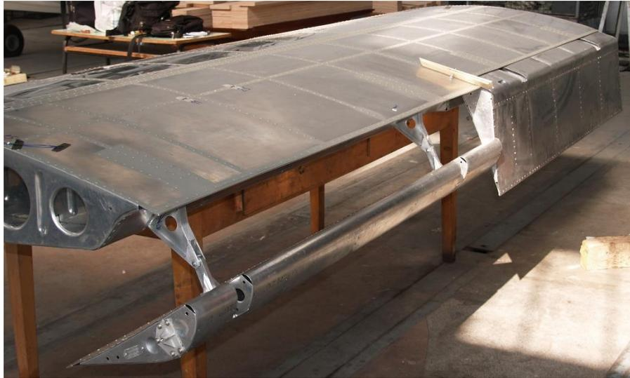
Figure 6.2 Completely functional flap and aileron
