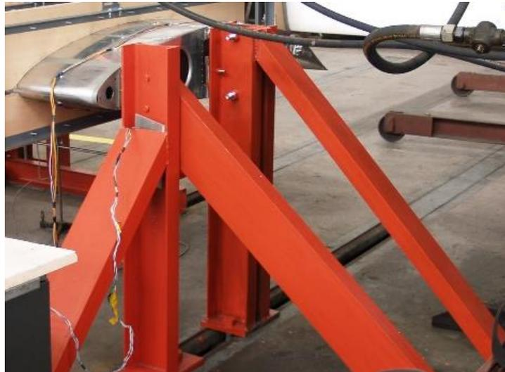
Figure 6.5 Test bench consisting of 6 I-beams carries the wing prototype during experiments
