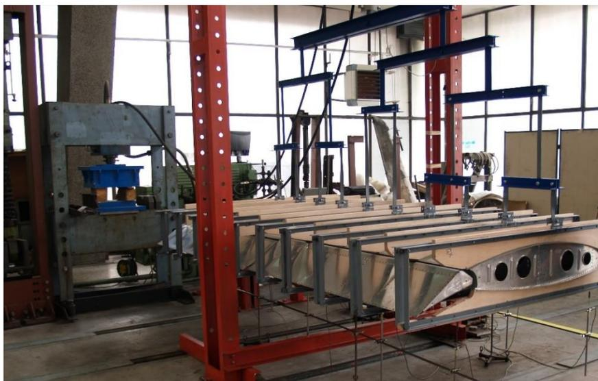
Figure 6.19 Test assembly for the light aerobatic aircraft wing (view from the other side)
