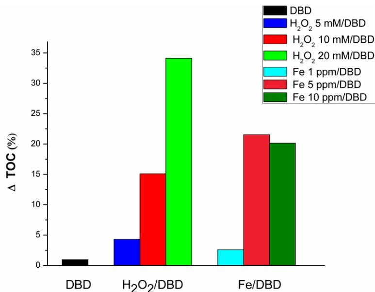
**Figure 33.** Mineralization efficiency after Triton x-100 degradation in the DBD reactor
