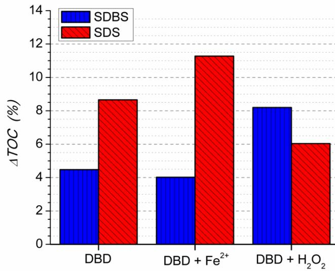
**Figure 45.** Mineralization efficiency of plasma treated solutions presented as percentage decrease of TOC value compared to solutions that didn't undergo plasma treatment.
