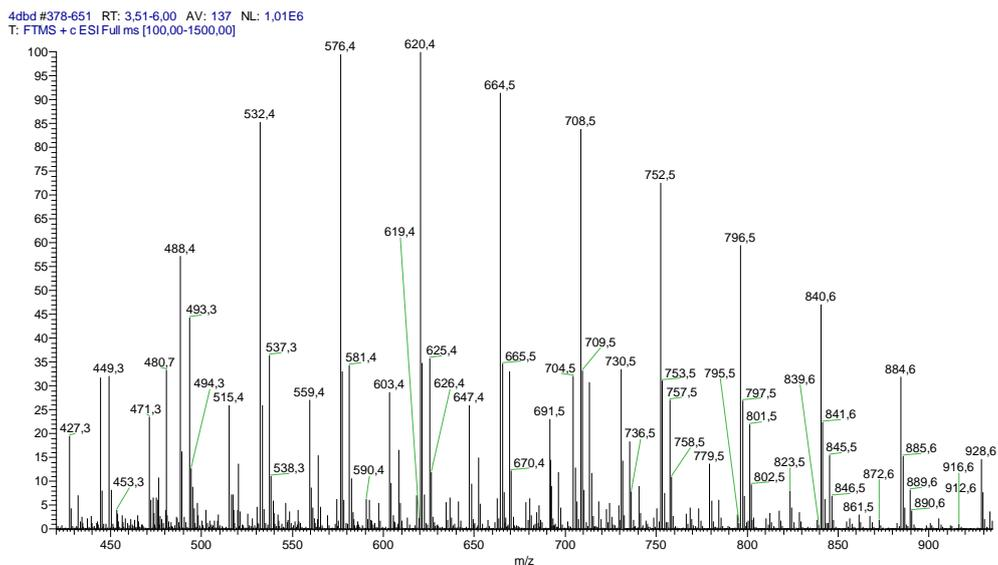
**Figure 29.** Mass spectrum of Triton X-100 solution after degradation in the non-catalytic DBD with introduced energy density of  $180 \text{ kJ L}^{-1}$
