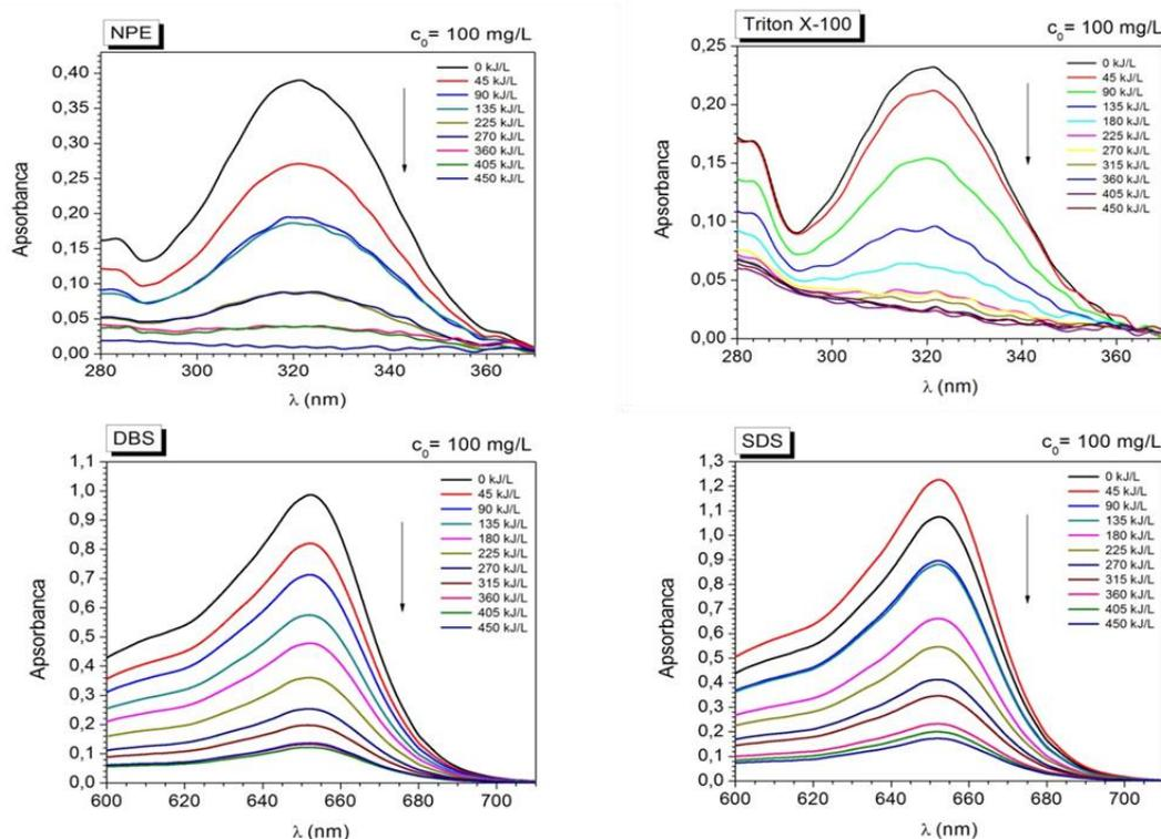
**Figure 21.** The changes in the UV-visible absorption spectra of the derivatized surfactant solution with different energy density introduced.
