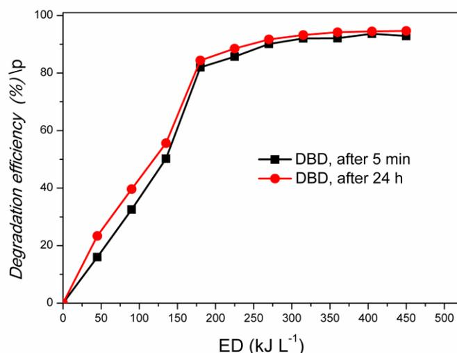
**Figure 22.** Degradation efficiency of TX-100 in DBD reactor after 5 min and 24 h.
