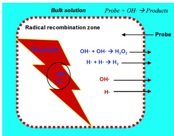
**Figure 15.** Various reaction zones involved in the production and reactions of reactive species formed by the high voltage electrical discharge in water. [146]
