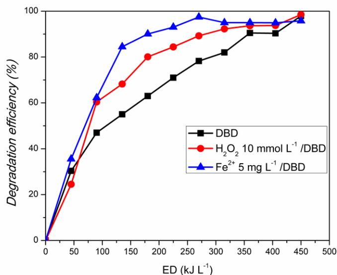
**Figure 26.** Degradation efficiency of NPE in the DBD reactor with catalyst and without catalyst
