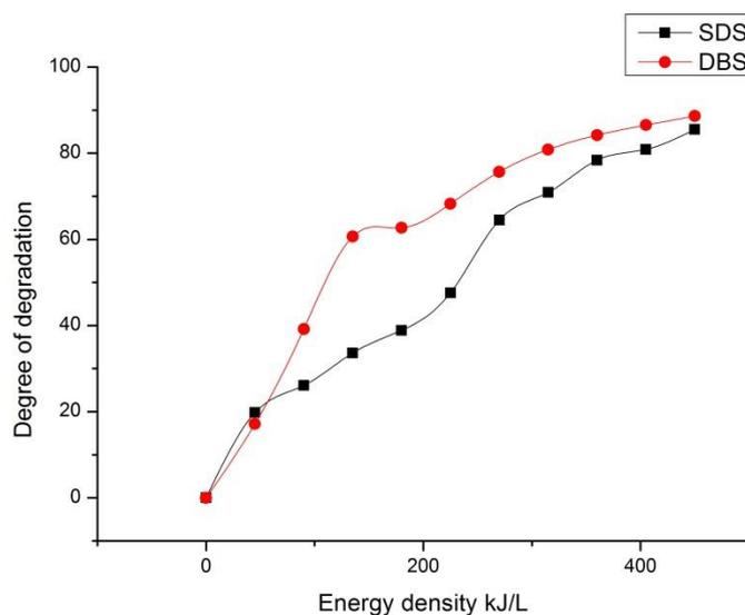
**Figure 34.** Degradation efficiency of SDBS and SDS with dielectric barrier discharge.
