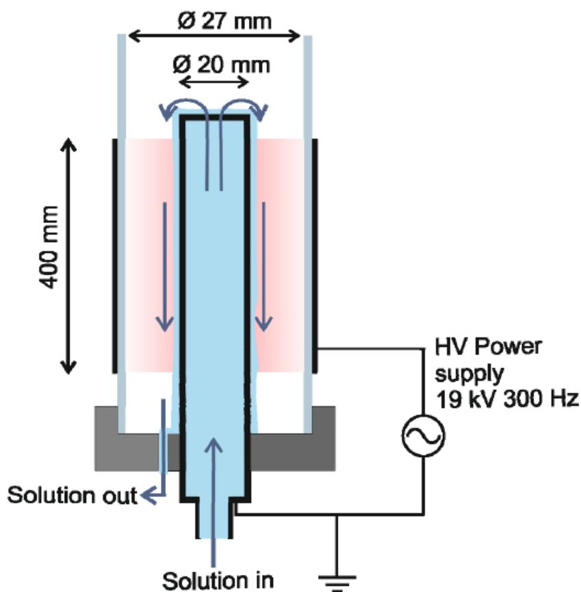
**Figure 19.** Water falling film dielectric barrier discharge (DBD) reactor used in the experiments.
