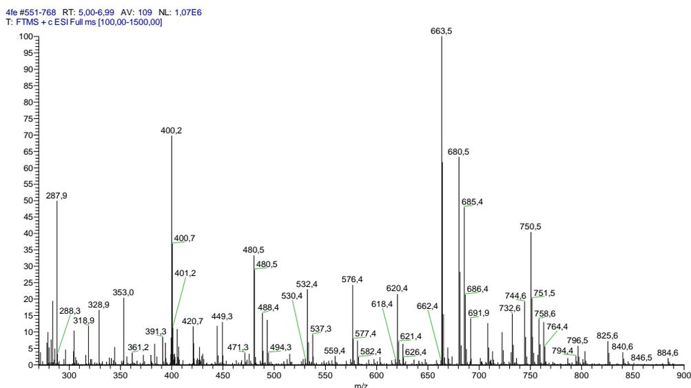
**Figure 30.** Mass spectrum of Triton X-100 solution after degradation in the  $\text{Fe}^{2+}$  DBD system with introduced energy of  $180 \text{ kJ L}^{-1}$
