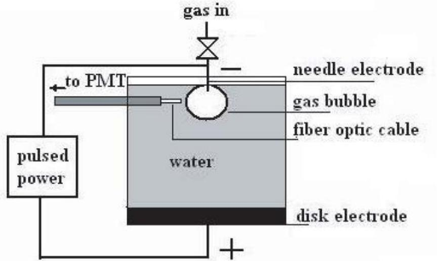
**Figure 17.** Schematic diagram of the bubble – water arrangement showing the bubble around the needle electrode with the disk electrode immersed in water. Gas is fed through the needle and a stationary bubble forms surrounding the tip of the needle [149].
