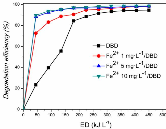
**Figure 25.** Degradation efficiency of TX-100 in the DBD reactor with the addition of  $\text{Fe}^{2+}$ .
