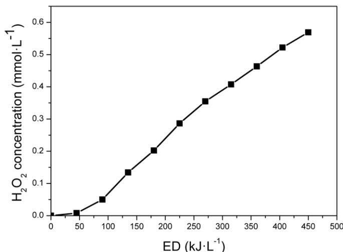
**Figure 24.** Production of H<sub>2</sub>O<sub>2</sub> in the DBD reactor with different ED values
