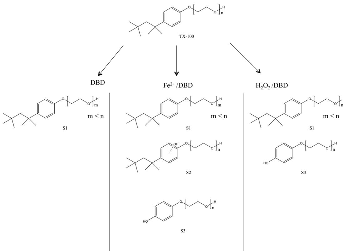
**Figure 27.** Degradation scheme of TX-100 decomposition with non-catalytic and catalytic DBD treatments.
