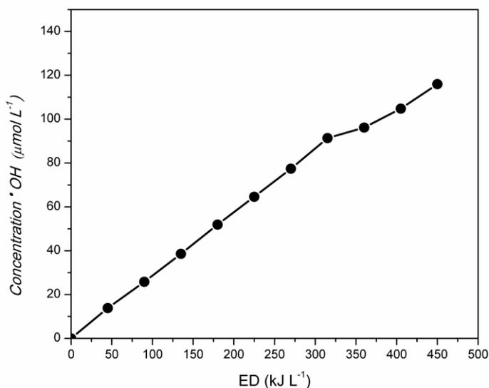
**Figure 38.** Changes in concentrations of hydroxyl radical in distilled water with introduced energy density
