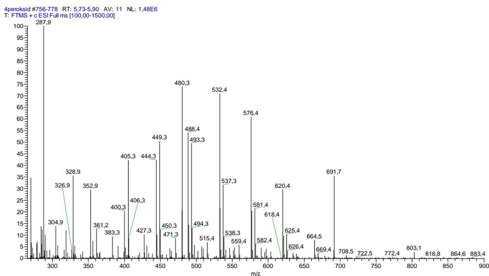
**Figure 31.** Mass spectrum of Triton X-100 solution after degradation in the H<sub>2</sub>O<sub>2</sub> /DBD system with introduced energy of 200 kJ L<sup>-1</sup>
