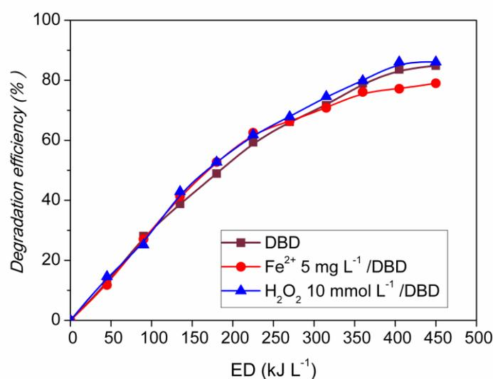
**Figure 42.** Degradation efficiency of SDS in DBD reactor.
