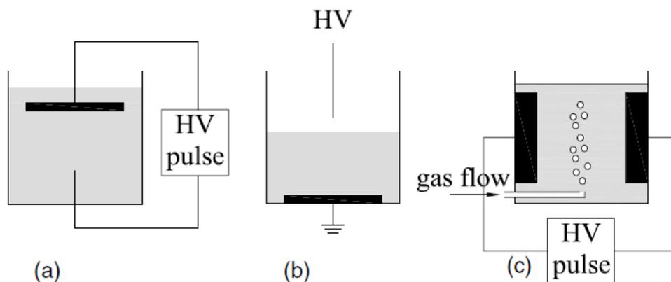
**Figure 14.** Typical electrode configurations for the three different types of discharges in contact with liquids. (a) Direct liquid phase discharge reactor (b) gas phase discharge reactor with liquid electrode (c) example of bubble discharge reactor [143].
