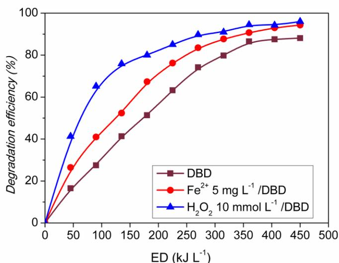
**Figure 41.** Degradation efficiency of SDBS in DBD reactor.
