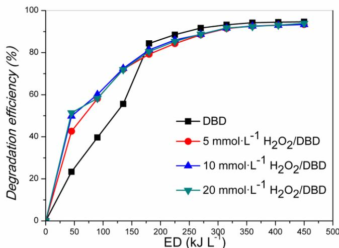
**Figure 23.** Degradation efficiency of TX-100 in the DBD reactor with the addition of H<sub>2</sub>O<sub>2</sub>.
