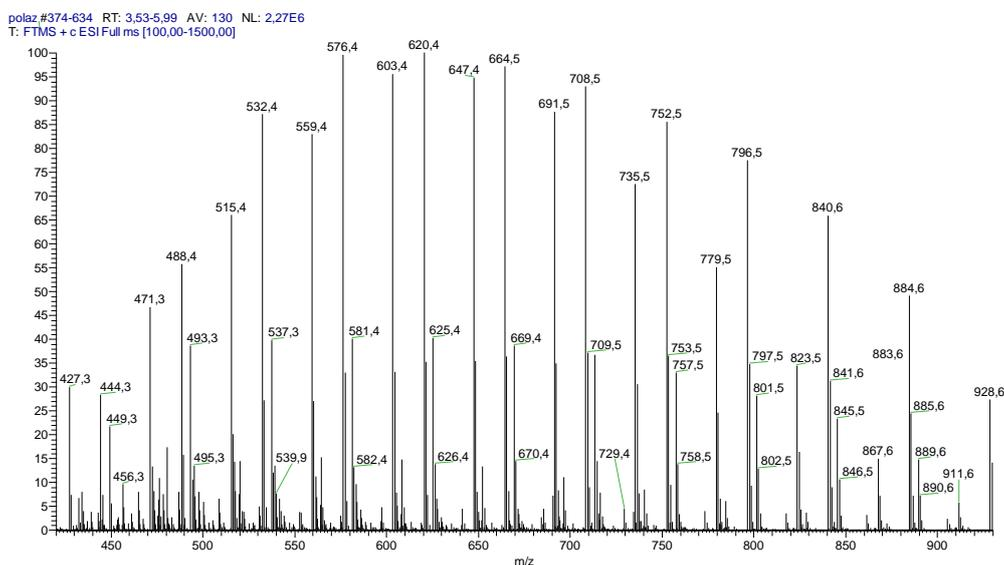
**Figure 28.** Mass spectrum of Triton X-100 molecules
