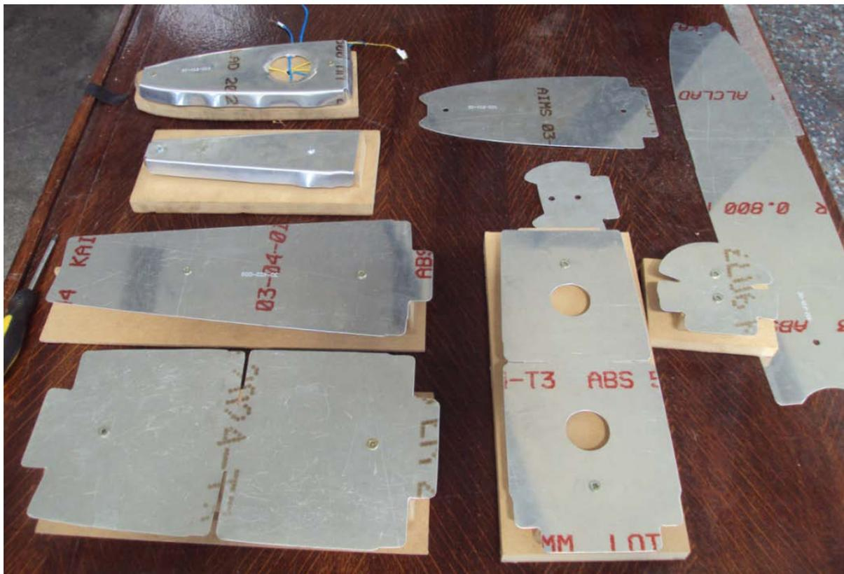
Figure8. 15: Blanks fixed in tools for experiments
