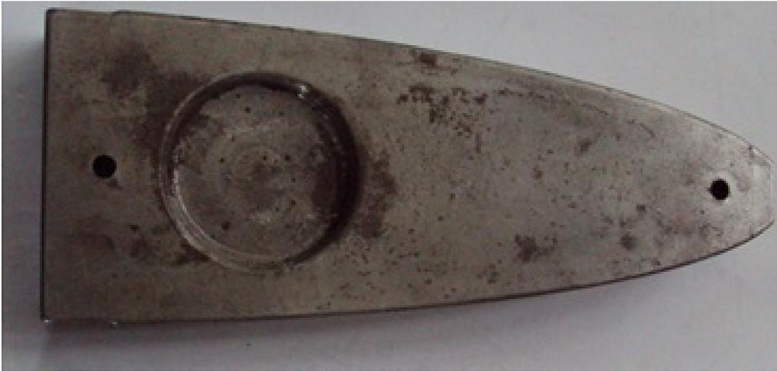
Figure 8. 21: New steel tool for rib with lightening hole
