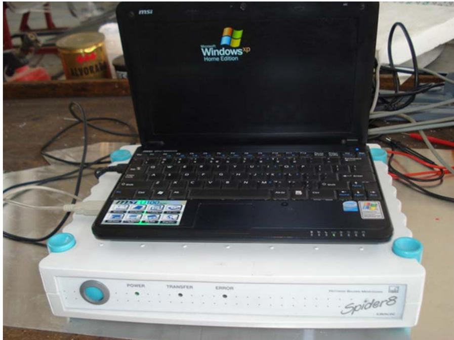
Figure8. 7:Spider8 acquisition system
