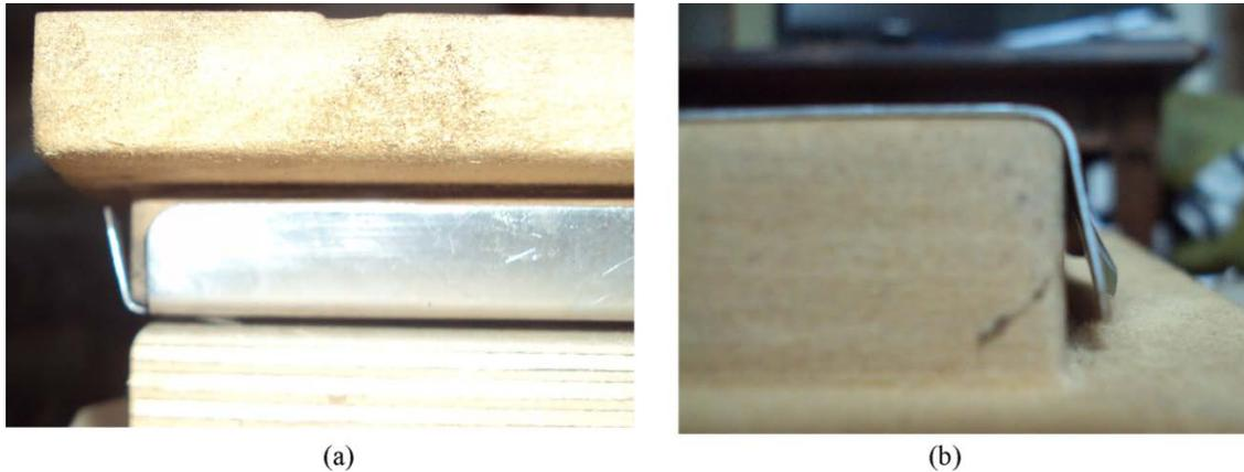
Figure8. 17: Springback in two ribs formed by rubber pad
