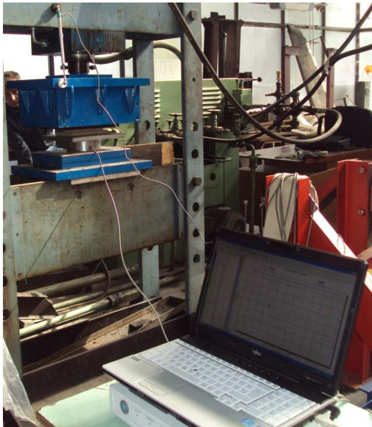
Figure8. 1: Hydraulic press machine and experimental rubber pad forming set-up
