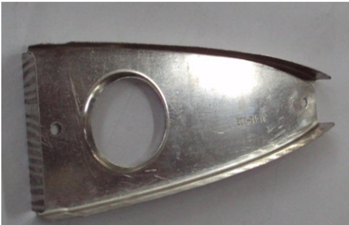
Figure 8. 22: Rib with lightening hole formed on steel tool
