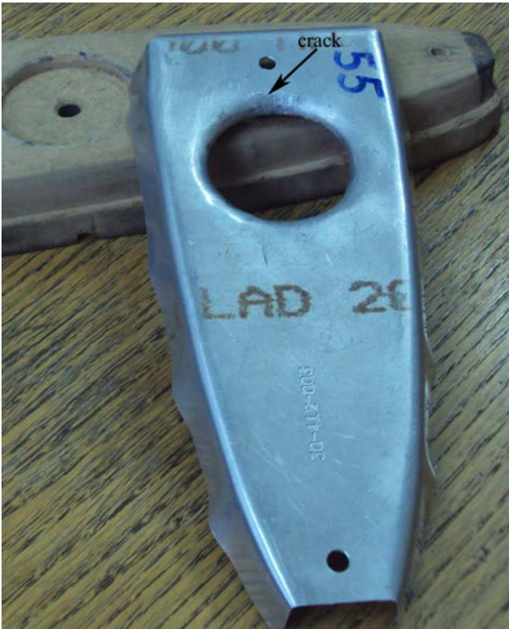
Figure8. 19: Small crack initiated in area with outer radius  $R_{II}$
