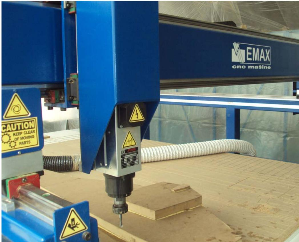
Figure8. 9: CNC machine used for wooden tools manufacturing
