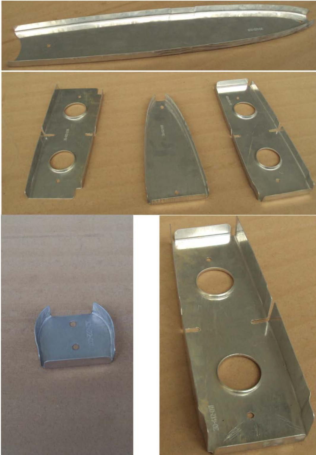
Figure8. 23: Several horizontal tail ribs manufactured on steel tools
