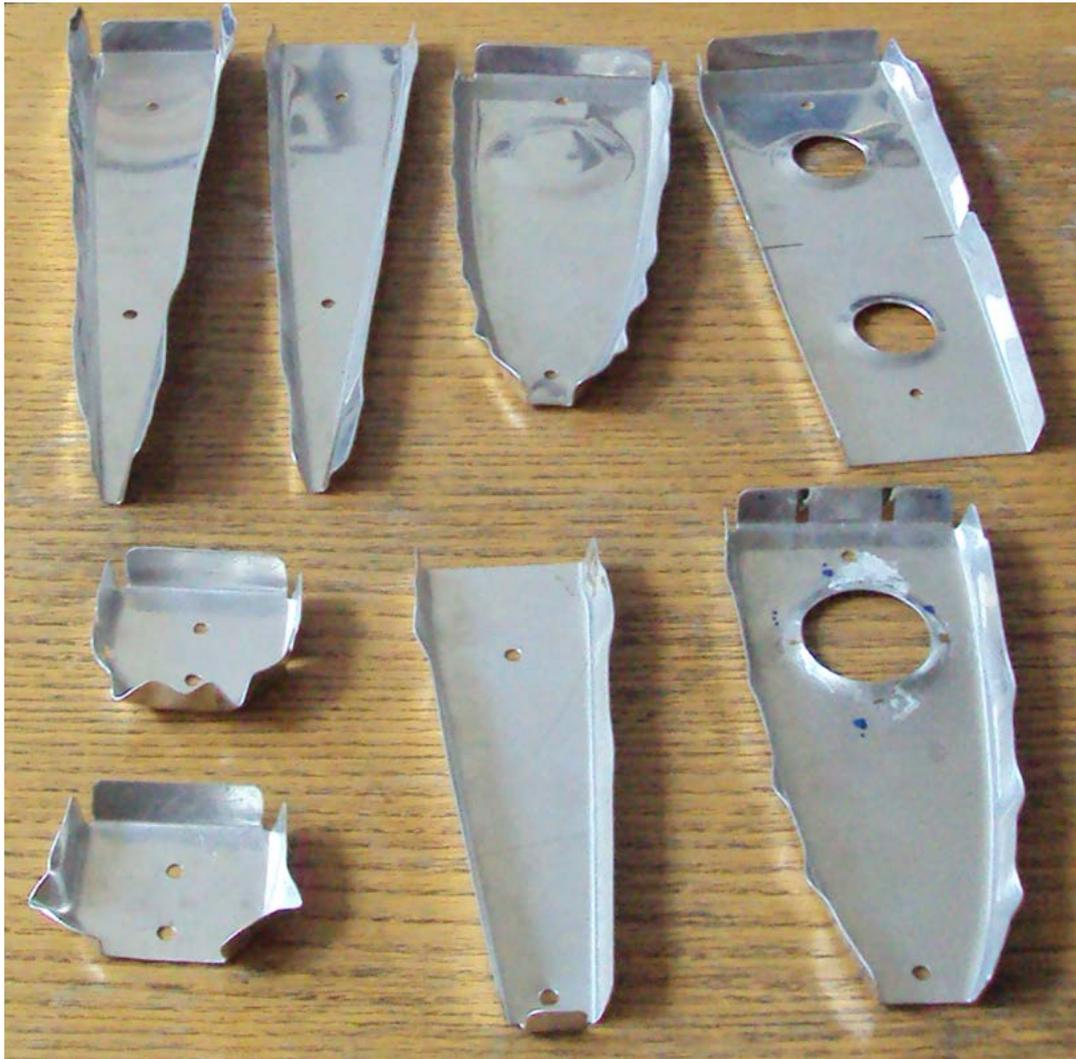
Figure8. 16: Shapes of ribs formed by rubber pad on experimental set-up
