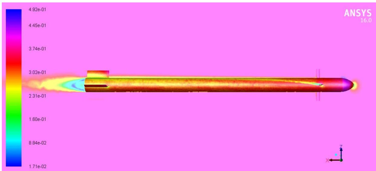
Figure 41 Mach number contours for 10 ° control deflection and angle of attack  $\alpha = 4^\circ$
