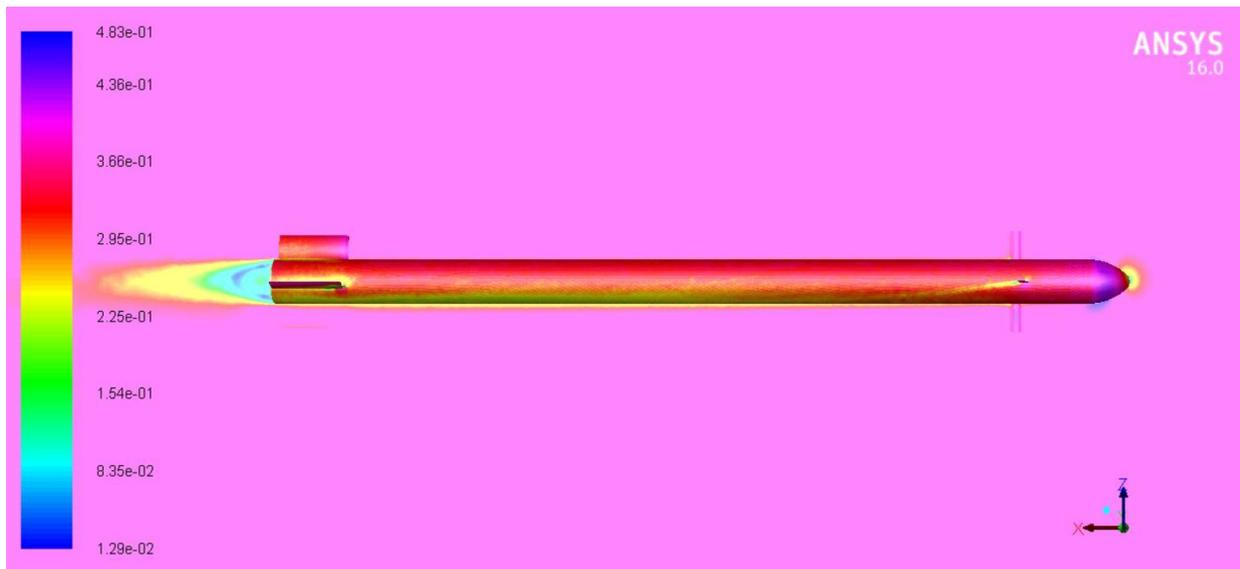
Figure 33 Mach number contours for 0 ° control deflection and angle of attack  $\alpha = -6^\circ$
