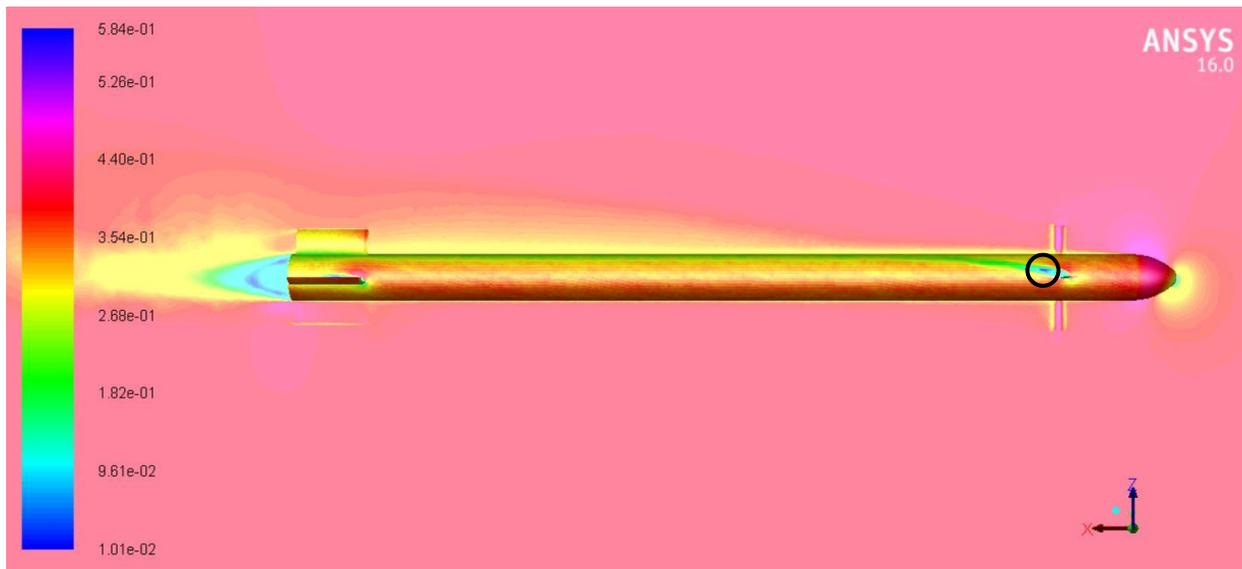
Figure 47 Mach number contours for 10 ° control deflection and angle of attack  $\alpha = 10^\circ$
