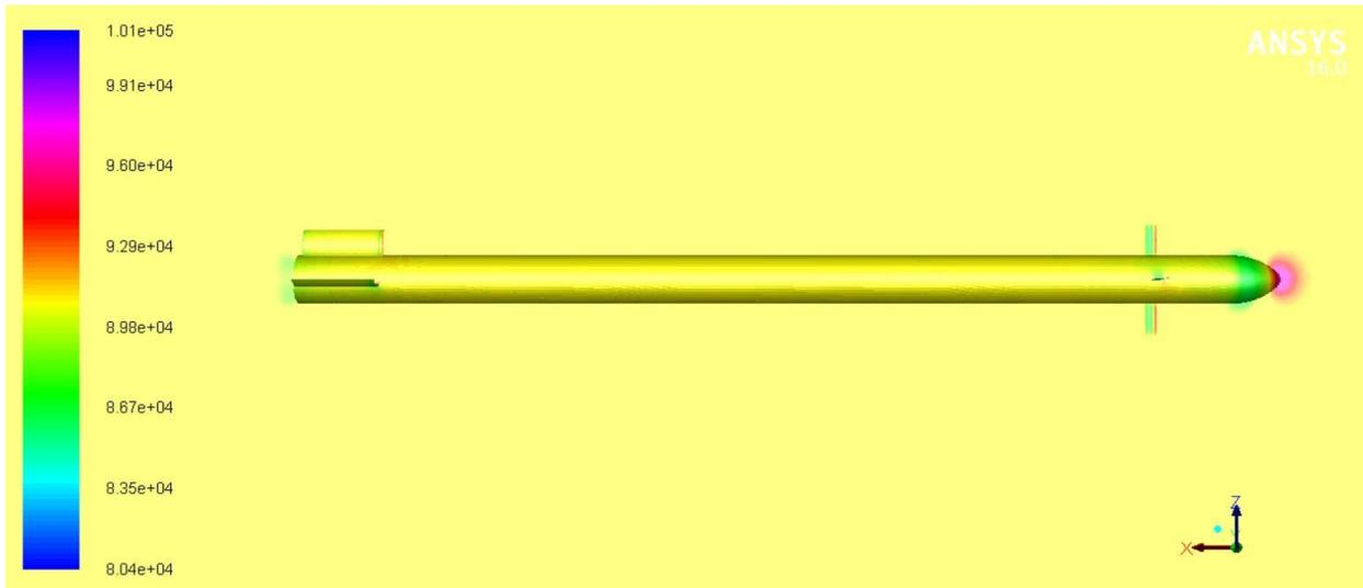
Figure 86 Static pressure contours for  $10^\circ$  control deflection and angle of attack  $\alpha = -2^\circ$
