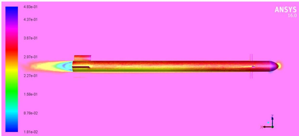
Figure 31 Mach number contours for  $0^\circ$  control deflection and angle of attack  $\alpha = -4^\circ$
