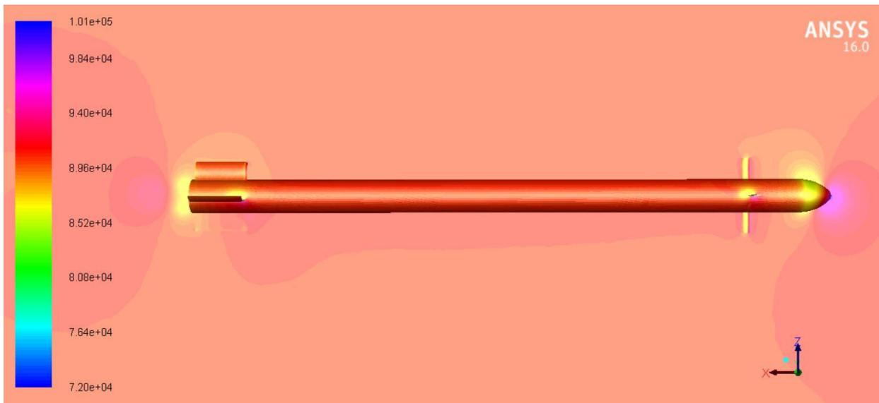
Figure 96 Static pressure contours for  $10^\circ$  control deflection and angle of attack  $\alpha = 8^\circ$
