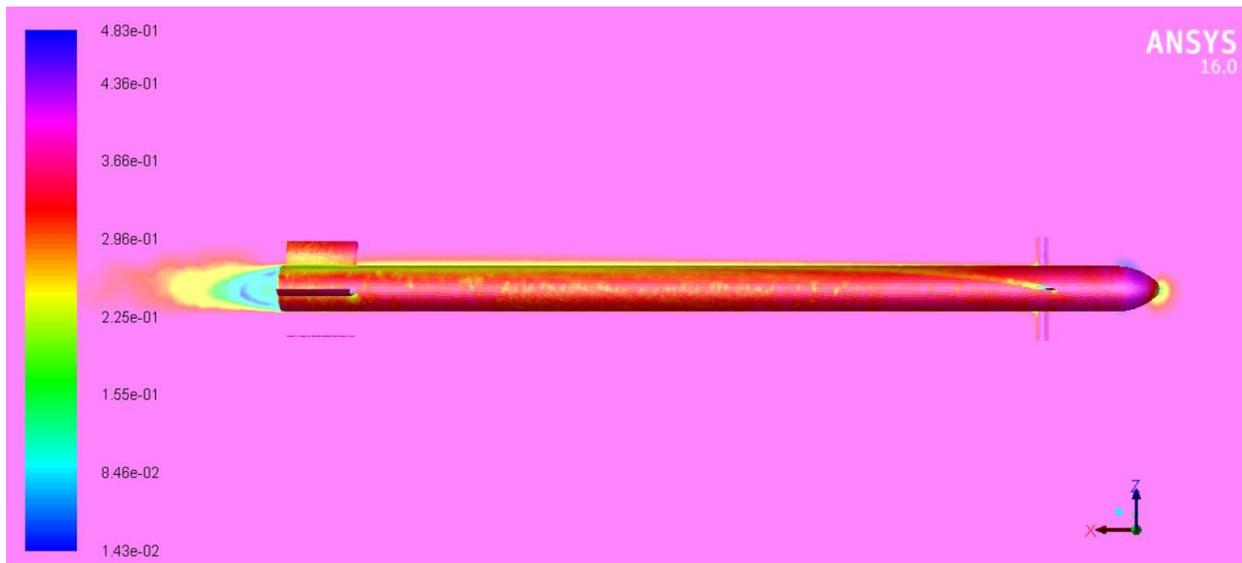
Figure 32 Mach number contours for 0 ° control deflection and angle of attack  $\alpha = 6^\circ$
