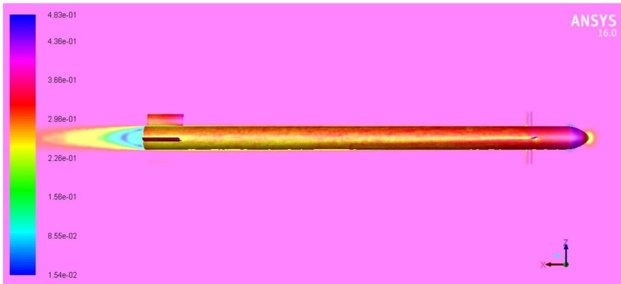
Figure 38 Mach number contours for 10 ° control deflection and angle of attack  $\alpha = 0^\circ$
