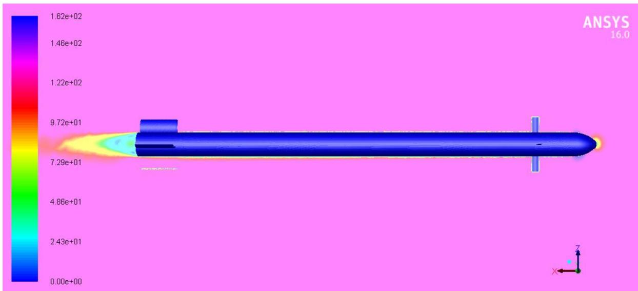
Figure 166 Velocity contours for 10 ° control deflection and angle of attack  $\alpha = -4^\circ$
