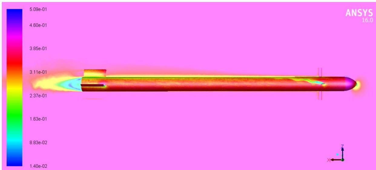
Figure 45 Mach number contours for 10 ° control deflection and angle of attack  $\alpha = 8^\circ$
