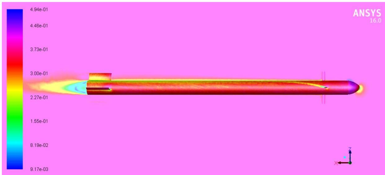
Figure 34 Mach number contours for  $0^\circ$  control deflection and angle of attack  $\alpha = 8^\circ$
