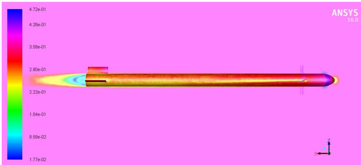
Figure 49 Mach number contours for 15 ° control deflection and angle of attack  $\alpha = 0^\circ$
