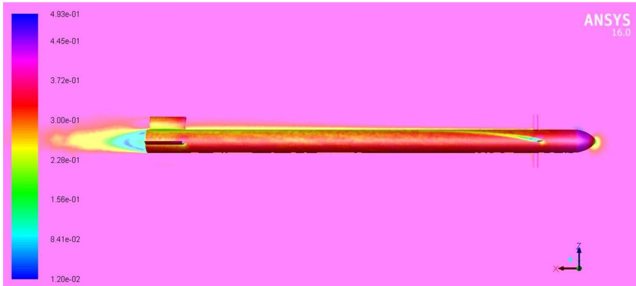
Figure 43 Mach number contours for 10 ° control deflection and angle of attack  $\alpha = 6^\circ$
