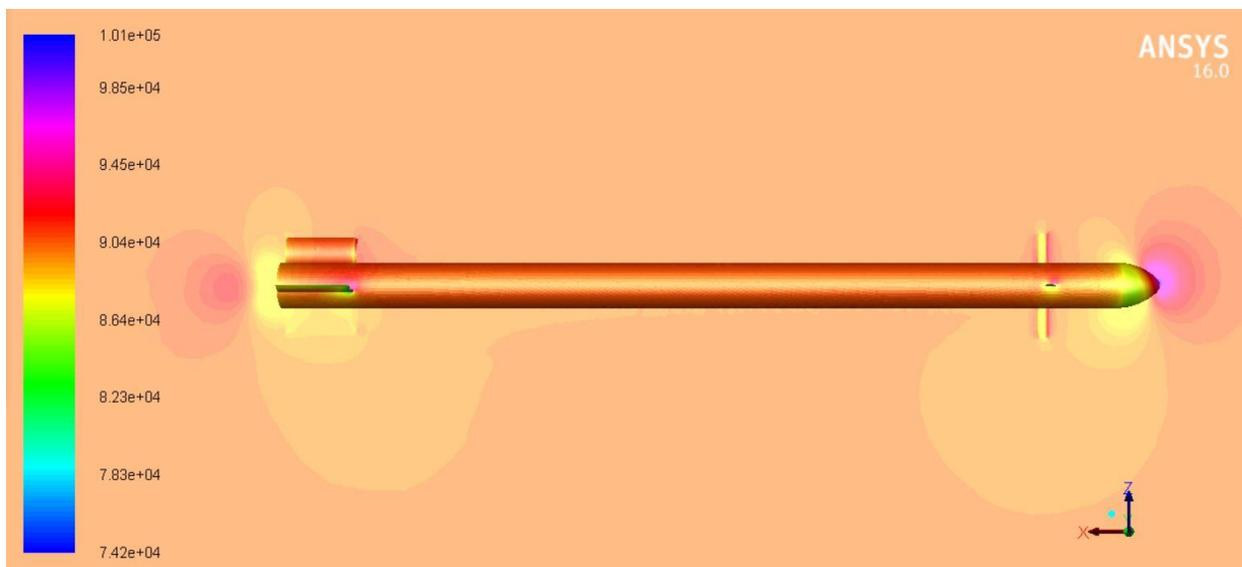
Figure 76 Static pressure contours for  $0^\circ$  control deflection and angle of attack  $\alpha = -8^\circ$
