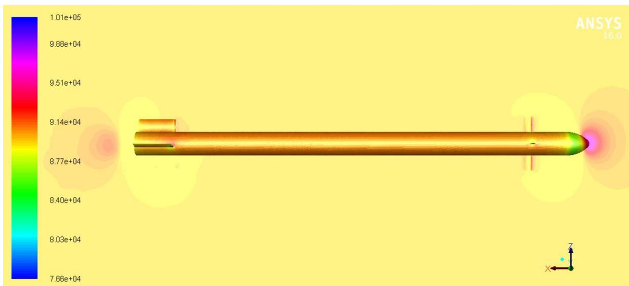
Figure 90 Static pressure contours for  $10^\circ$  control deflection and angle of attack  $\alpha = -4^\circ$
