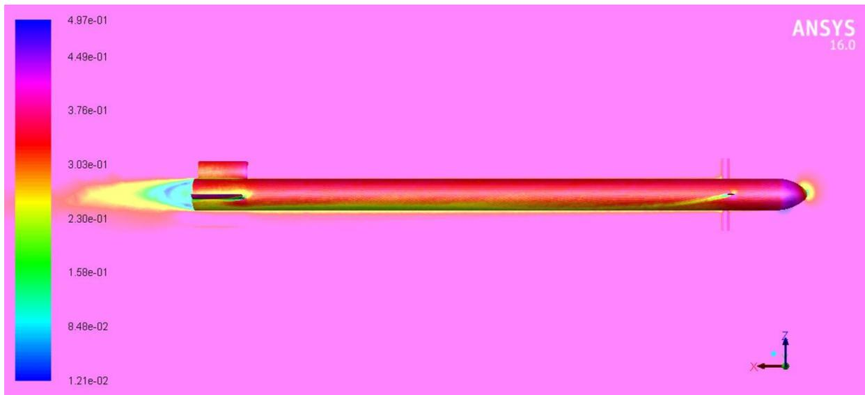
Figure 35 Mach number contours for 0 ° control deflection and angle of attack  $\alpha = -8^\circ$
