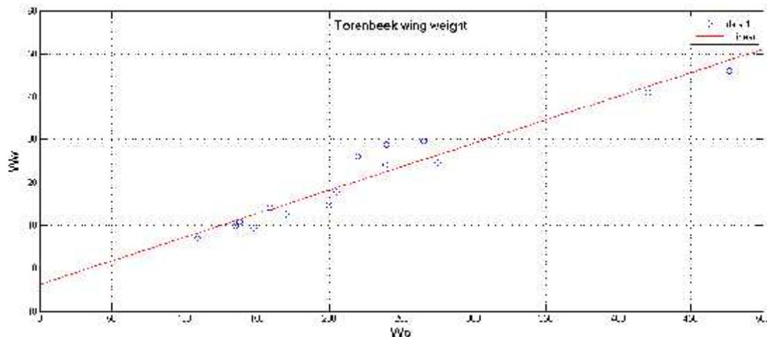
Figure (6-4) Torenbeek wing weight estimation
