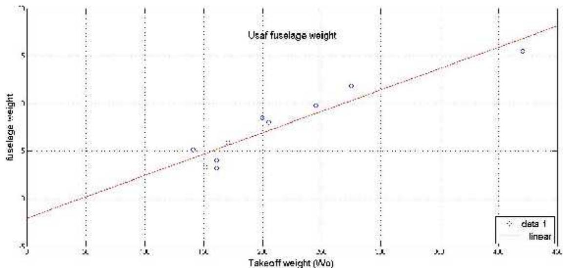
Figure (8-6) Usaf fuselage weight estimation
