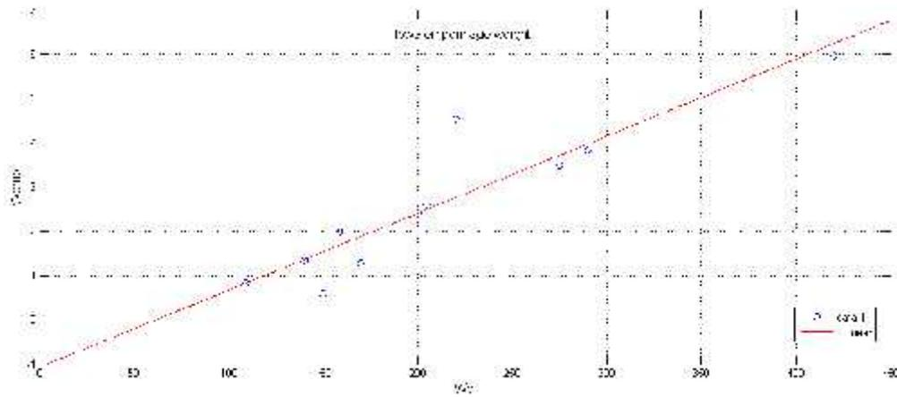
Figure (7-18) Howe empennage weight estimation
