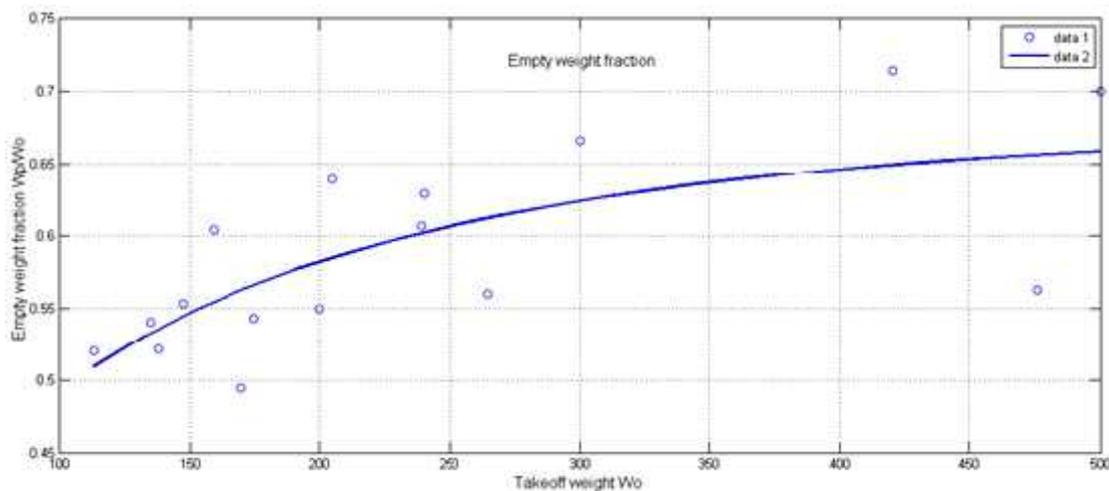
Figure (4-5) Empty weight fraction versus takeoff weight
