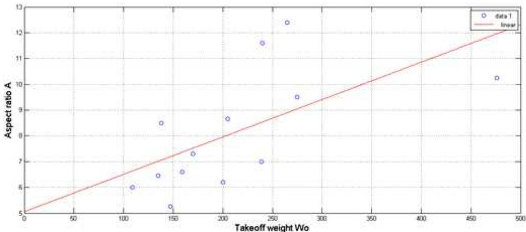
Figure (4-9) represents aspect ratio and takeoff weight relationship.
