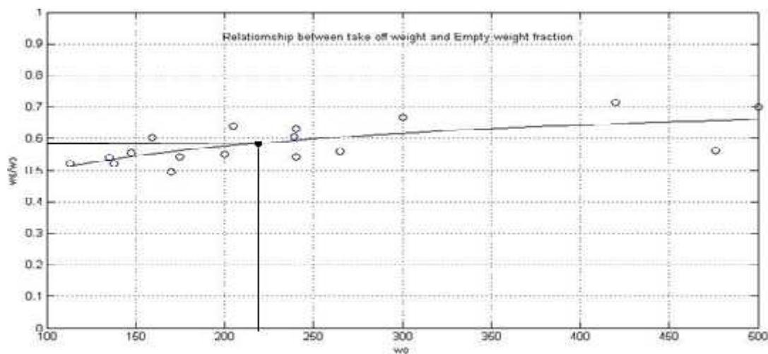
Figure (5-4) Empty weight fraction and takeoff weight relationship
