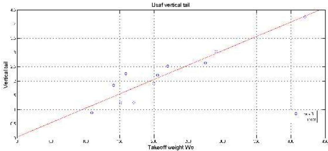
Figure (7-5) Usaf vertical tail weight estimation
