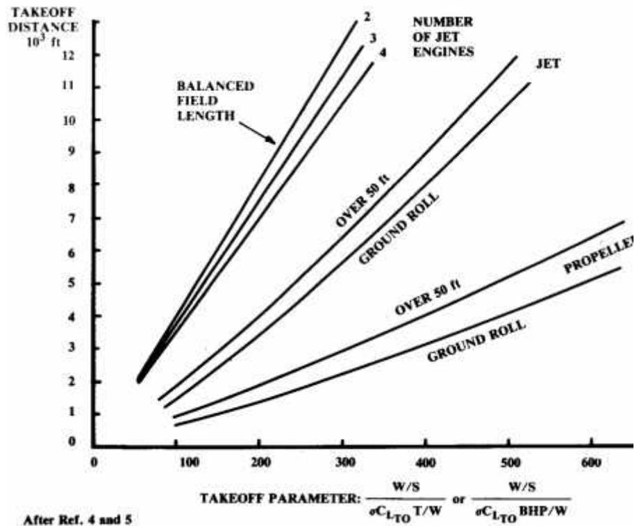
Figure (5-9) The relationship between takeoff parameter and takeoff distance
