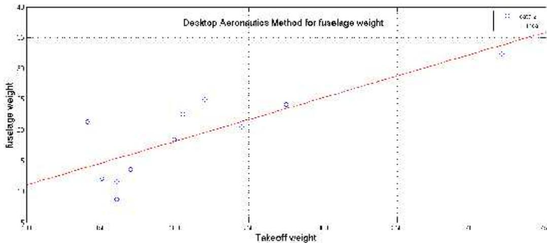
Figure (8-7) Kroo fuselage weight estimation
