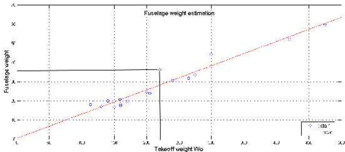
Figure (10-4) The new formula for fuselage weight estimation
