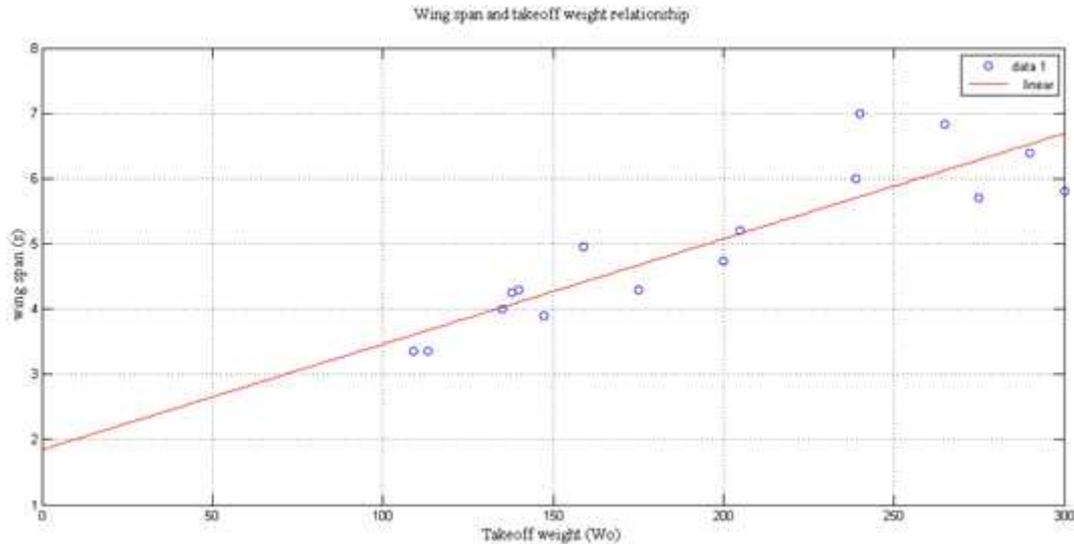
Figure (4-8) Wing span and takeoff weight relationship
