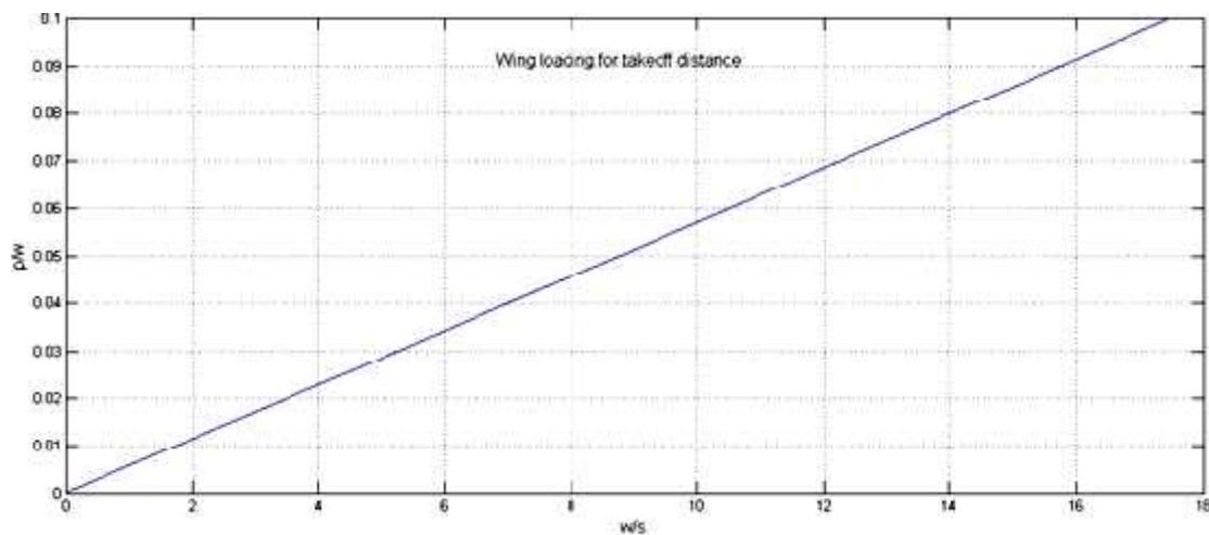
Figure (5-7) Wing loading and takeoff weight relationship
