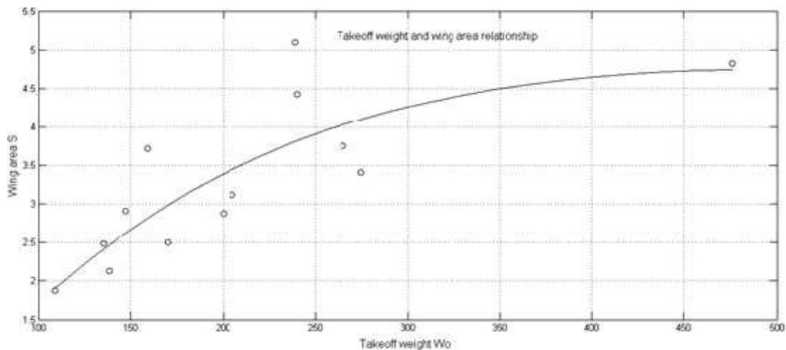
Figure(4-7) Wing area versus takeoff weight
