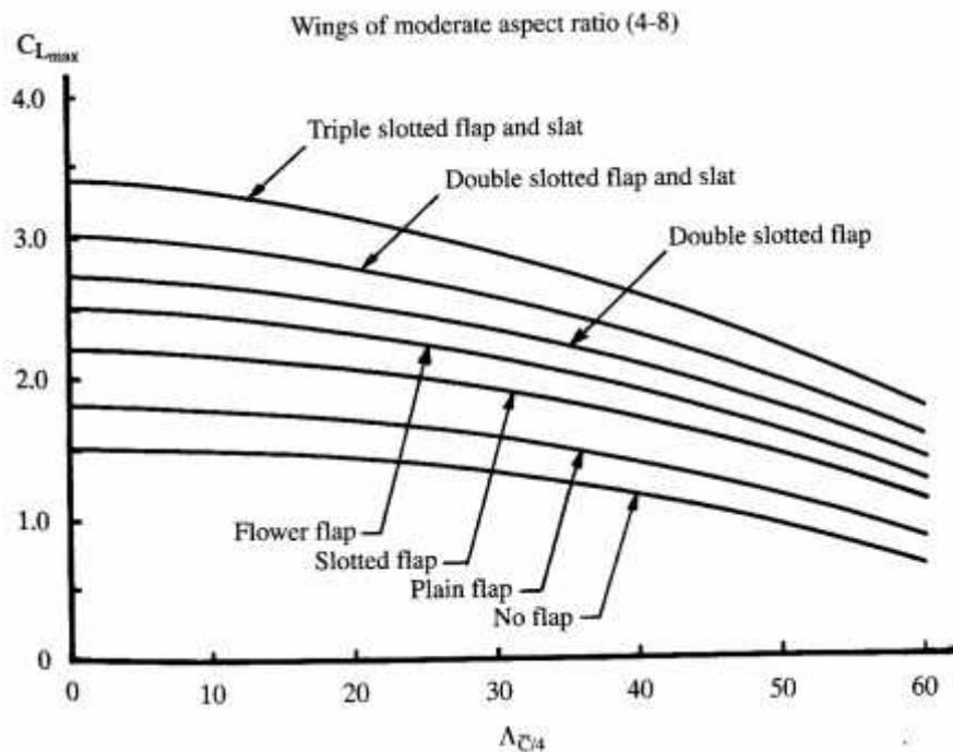
Figure (5-6) Maximum lift coefficient  $C_{Lm}$  value for different sweep angle
