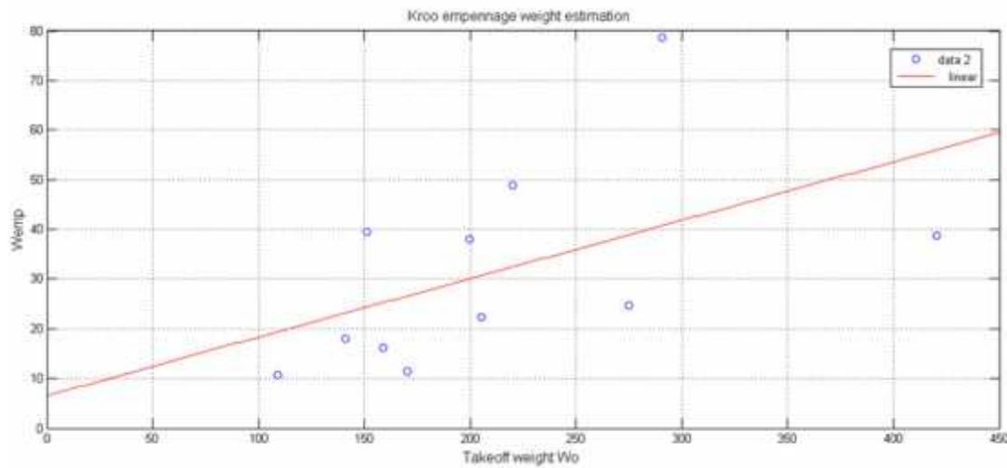
Figure (7-15) Kroo empennage weight estimation
