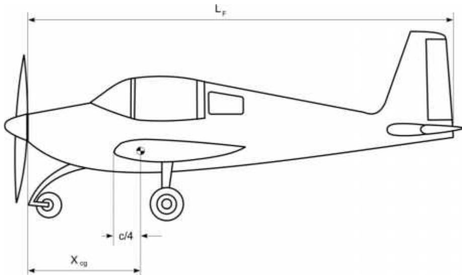
Figure (5-15) Aircraft sketch illustrates the fuselage length and the center of gravity
