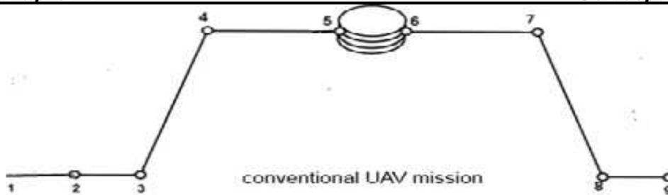
Figure (4-2) mission profile for conventional UAV
