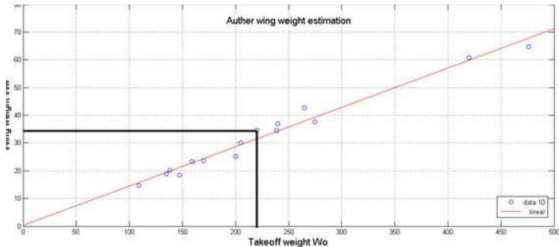
Figure (10-3) The new formula for wing weight estimation
