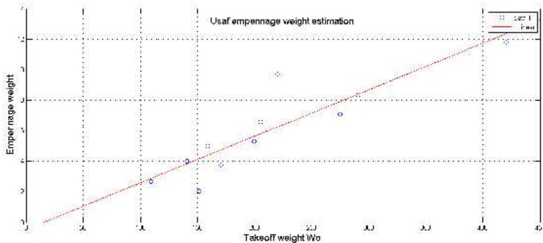
Figure (7-6) Usaf empennage weight estimation
