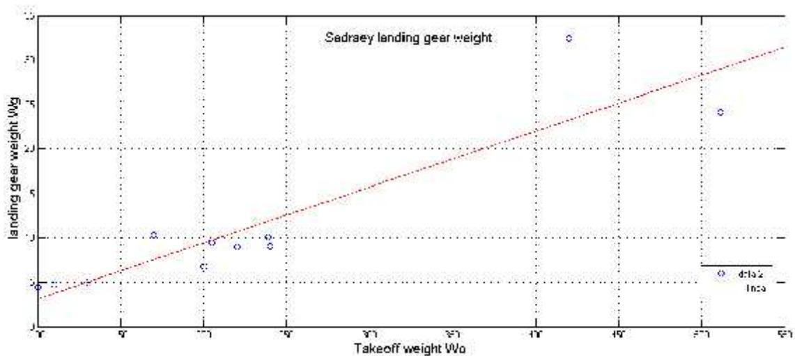
Figure (9-4) Sadraey landing gear weight estimation
