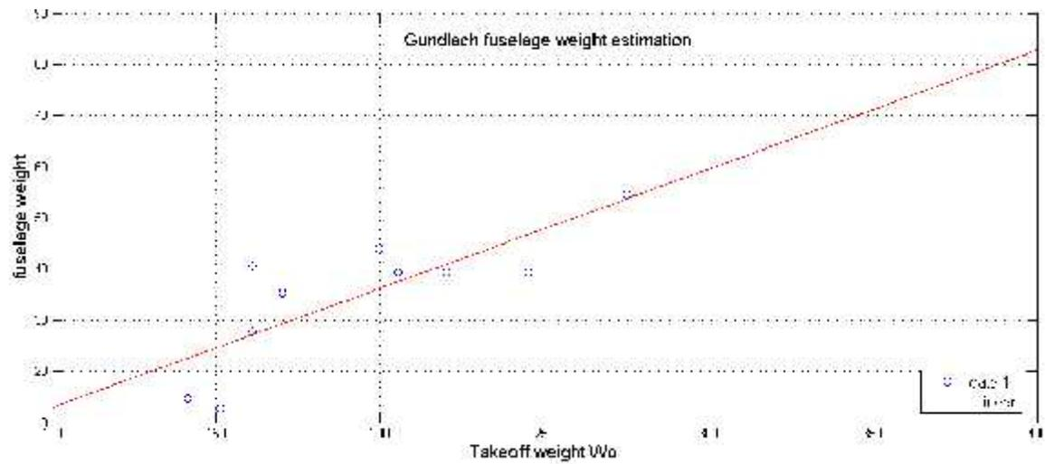
Figure (8-8) Gundlach fuselage weight estimation
