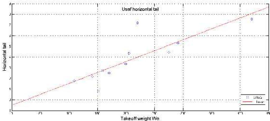
Figure (7-4) Usaf horizontal tail weight estimation
